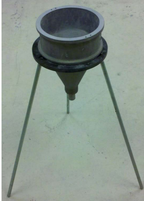
Figure 5—Flow cone used to determine rheological properties of grout in the field. See ASTM C939 for dimensions
