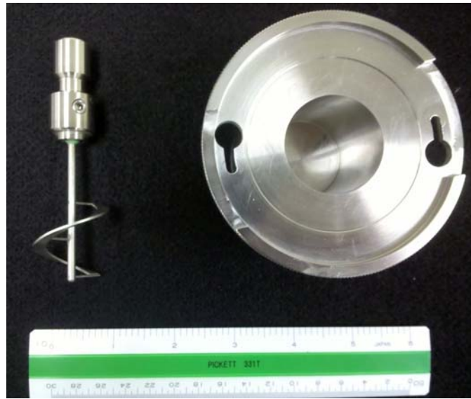
Figure 19—Helical ribbon (left) and cup (right) DSR geometry
