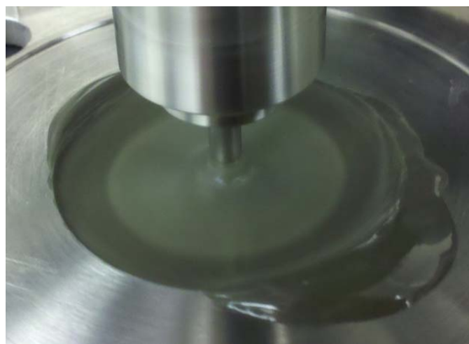
Figure 48—Segregation observed in PT grout during 60-min NSR viscosity test
