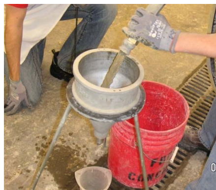
Figure 9—Preparation for modified flow cone test
