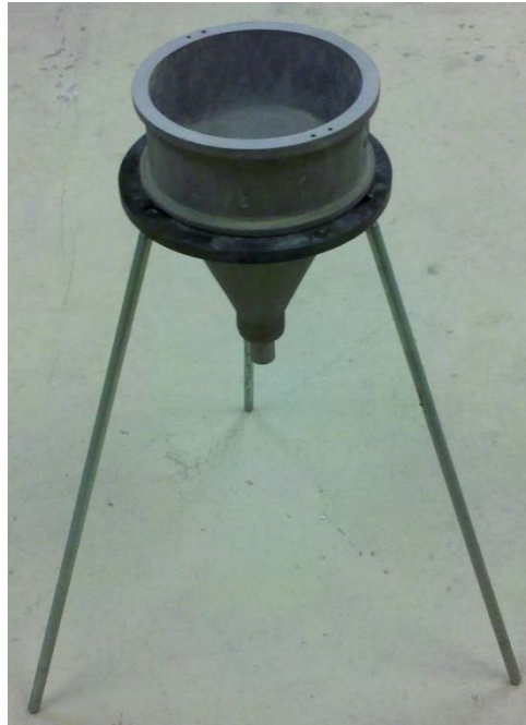
Figure 5—Flow cone used to determine rheological properties of grout in the field. See ASTM C939 for dimensions
