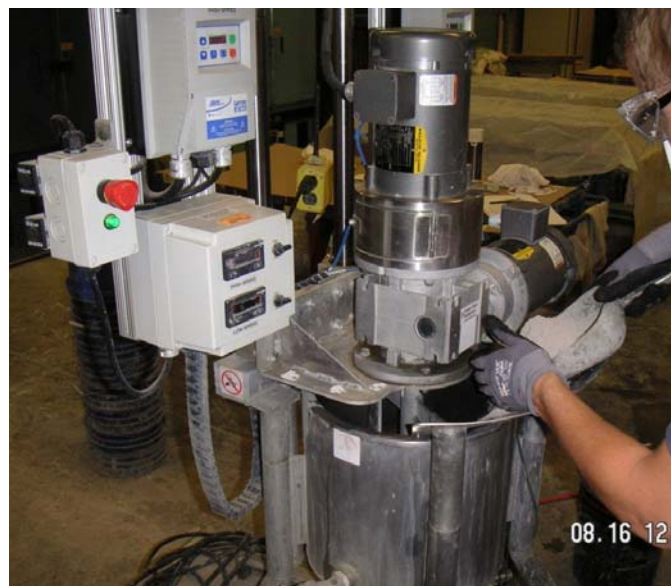
Figure 12—Add dry material to mixer over a period of 3 min to 5 min
