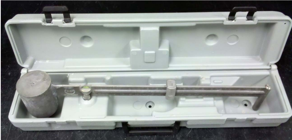
Figure 35—Mud balance used to determine wet density of grout samples during HTGF testing
