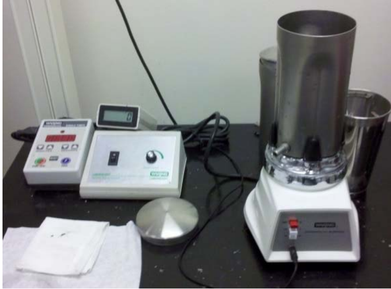
Figure 14—Waring HGBTAC30 commercial blender used for mixing
