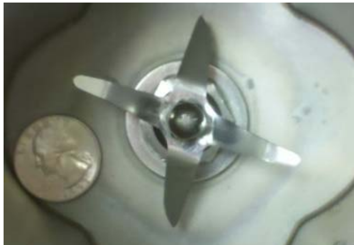
Figure 15—Blade configuration used in mix procedure with quarter shown for reference
