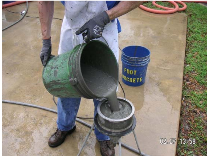
Figure 34—Flow cone used to determine fluidity of grout samples during HTGF testing
