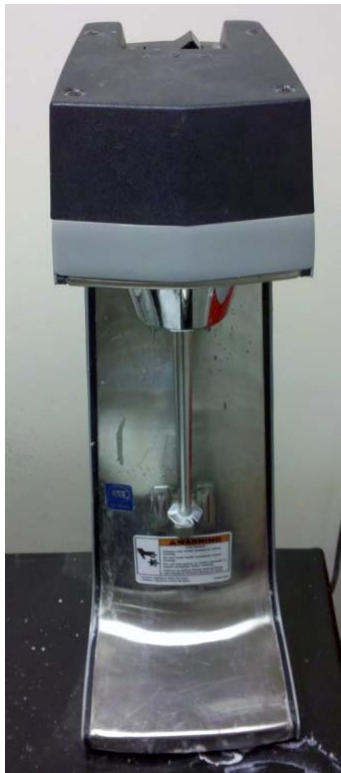
Figure 16—Plunger mixer used to agitate grout before testing
