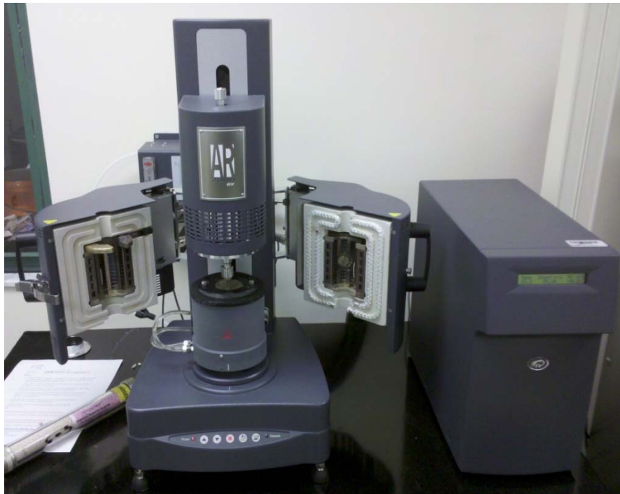
Figure 17—Dynamic Shear Rheometer with helical ribbon and cup geometry
