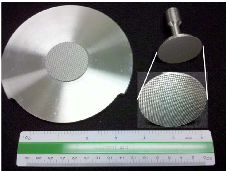
Figure 18—Serrated parallel plate DSR geometry – bottom plate (left) and top plate (right)
