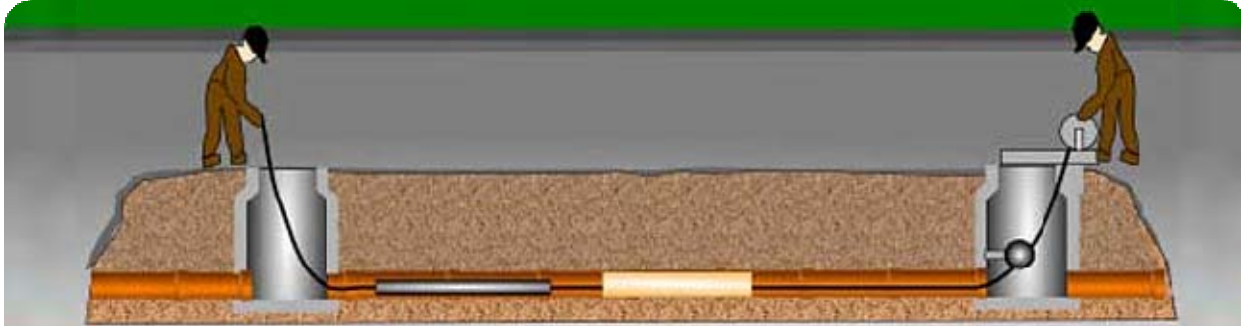
Figure 2-21. Point repair using cured-in-place pipe method (Perma-Liner Industries 2010).
