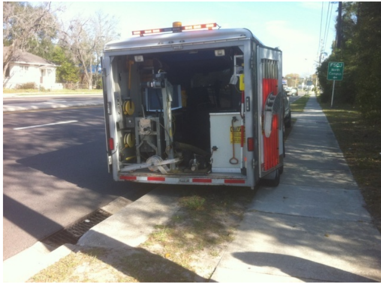
Figure 3-1. District 2 trailer equipped with CCTV video – Pipe inspection crew inspecting a pipe connected to a curb and gutter inlet in Duval County.
