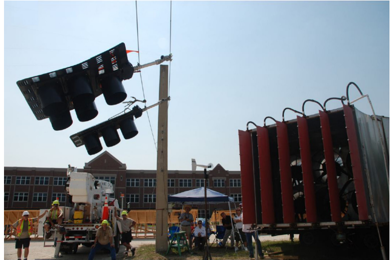
Dual signals are suspended from dual cables by rigid pipe hangers in this test setup. The signals are blown back to a high angle under the influence of the wind load generated by the UF Hurricane Simulator, partially visible at the right.
