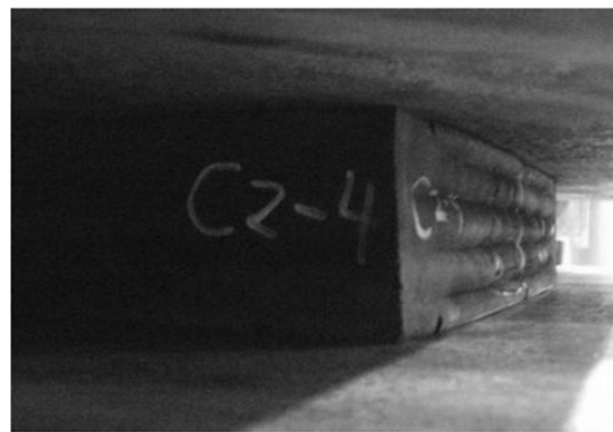
Figure 6.2 Bulging of neoprene layers under compression:
