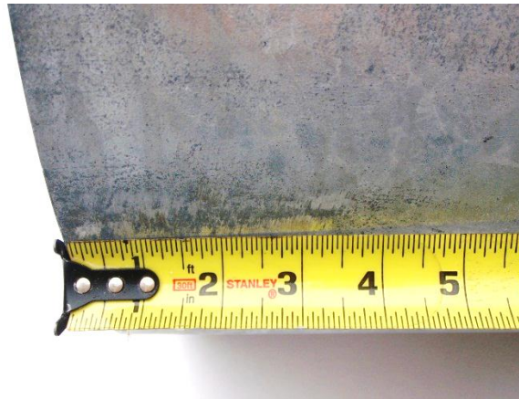
Figure 5-12. Scratches on the tension face of the inner pole. Photo courtesy of S. Dalton.
