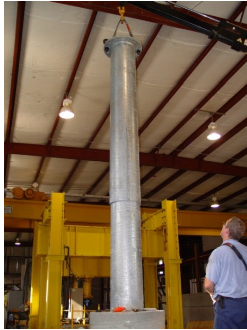
Figure 6-3. Placement of the upper pole for the test apparatus using an overhead lift. Photo courtesy of FDOT.
