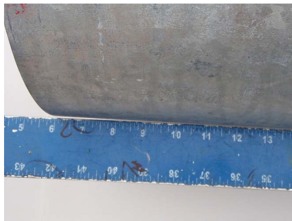
Figure 5-13. Plastic deformation on the tension face of the inner pole in slip joint region. Photo courtesy of S. Dalton.
