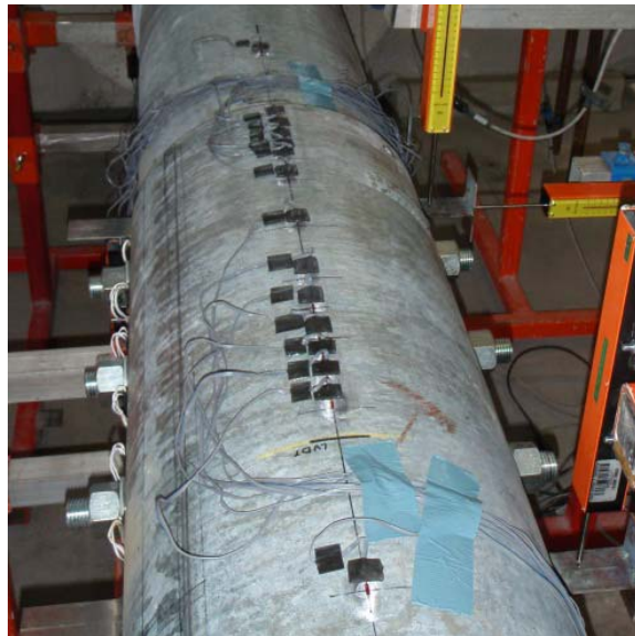
Figure 5-9. Flexural strain gauges on compression face of outer pole along the slip joint. Photo courtesy of S. Dalton.
