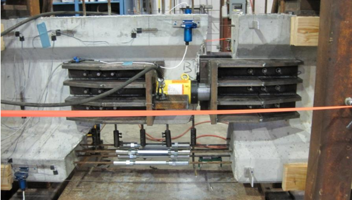
Figure 55—Splice stressed with lock-nuts engaged
