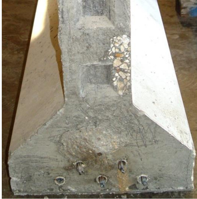
Figure 142–Post-test: End view of unbonded segment
