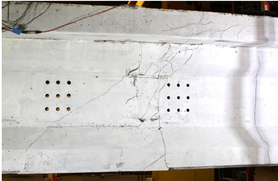
Figure 131–SU2: Joint at failure
