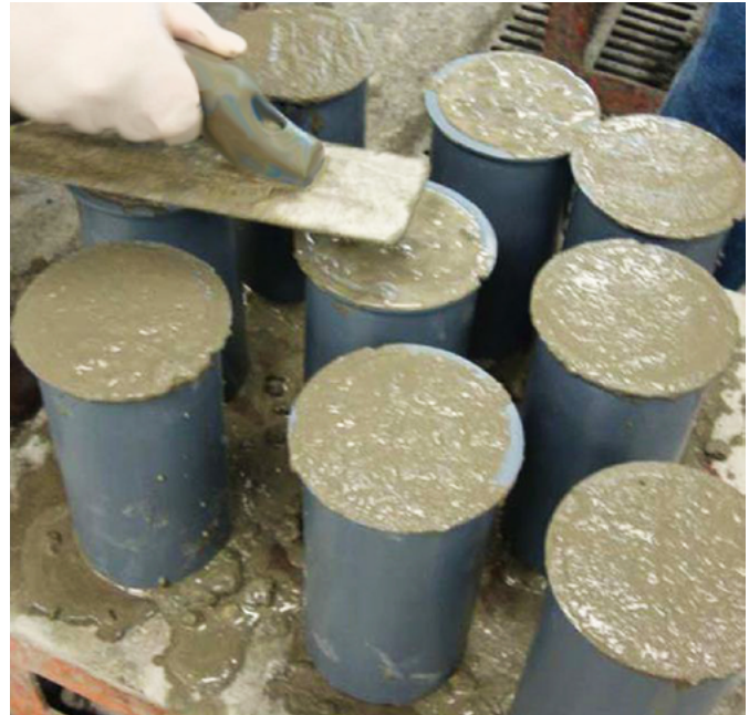
Concrete samples using a variety of aggregates are prepared for compression testing on the vibrating table.
