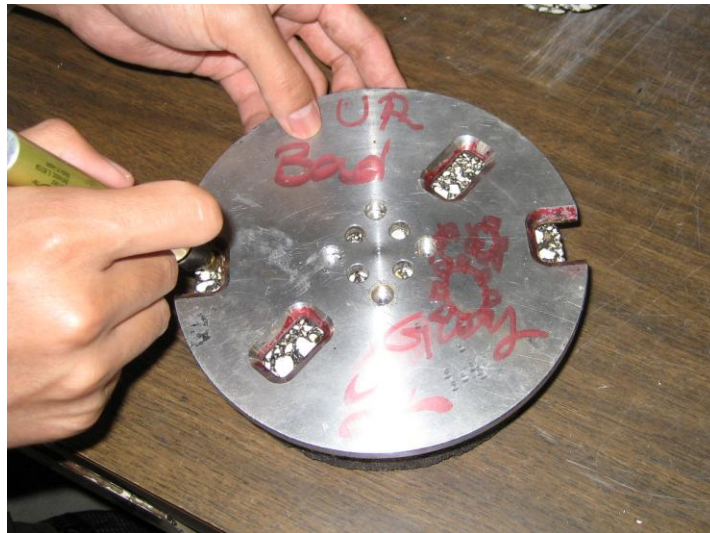
Figure 4-7 Marking the loading axis
