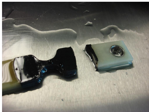
Figure 3-7 Geometry No. 3, asphalt peeled off from load head.
