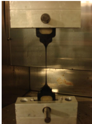
Figure 4-27 PG 82-22 at 15°C, extension greater than 1.2 in without fracture
