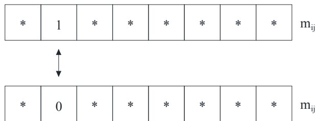
Figure A-1 Genetic algorithm: a) parameter coding, and b) crossover and mutation
