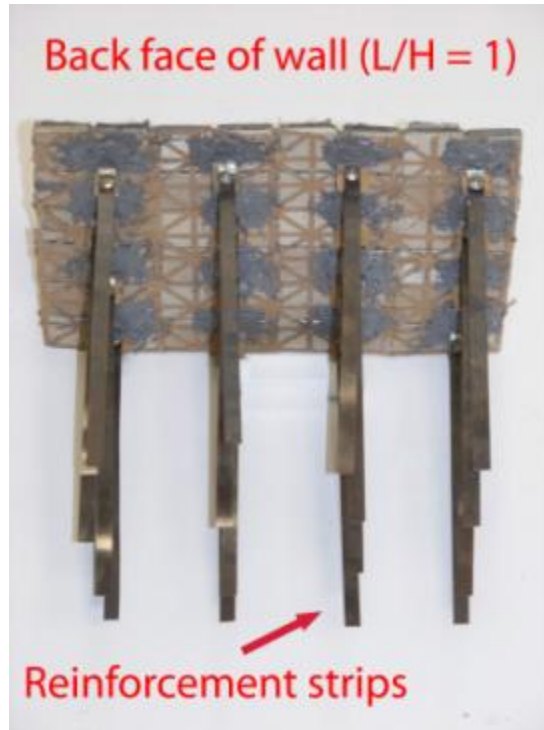
Figure 3-1 Rear view of MSE wall with reinforcement
