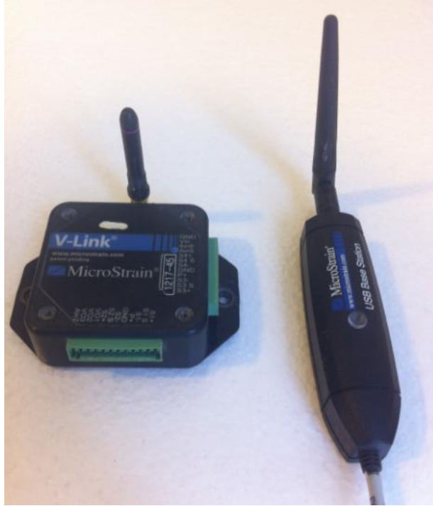
Figure 2-11 MicroStrain V-Link node and receiver
