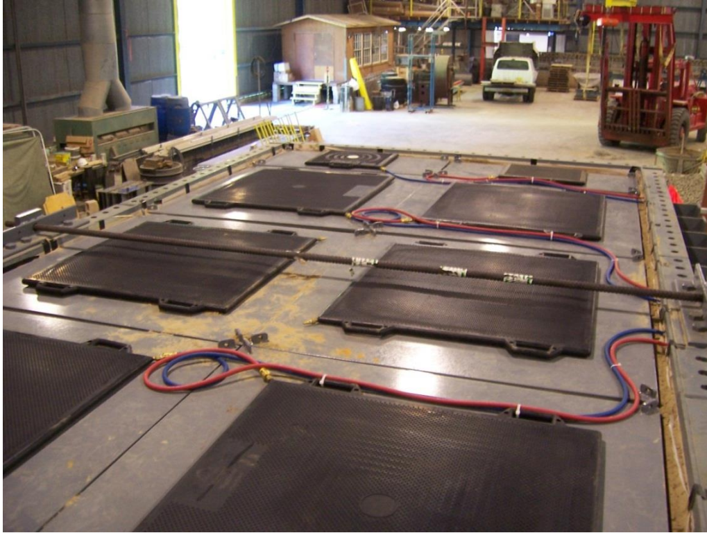
Figure 3-5. Installed loading mechanism.
