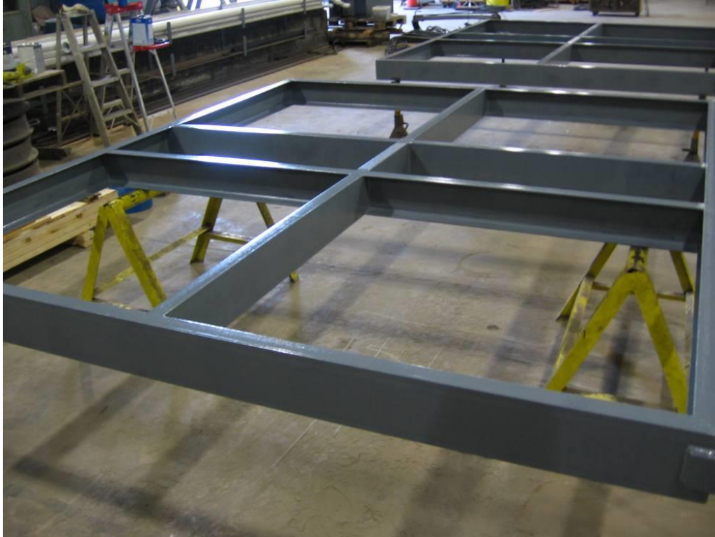
Figure 8-1. Painted trench box frames.
