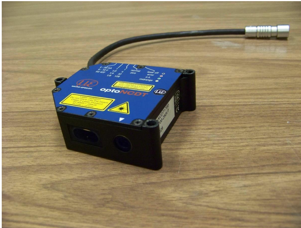
Figure 10-10. Purchased laser for 24 inch pipe testing
