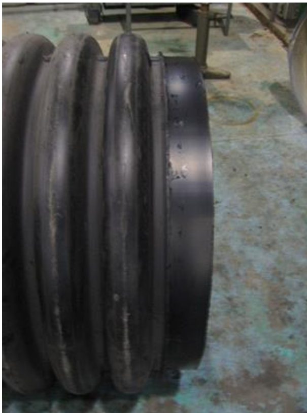
Figure 9-2. HDPE pipe end modification
