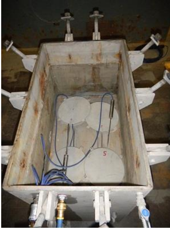
Figure 4-4. Earth pressure cells inside pressure vessel.
