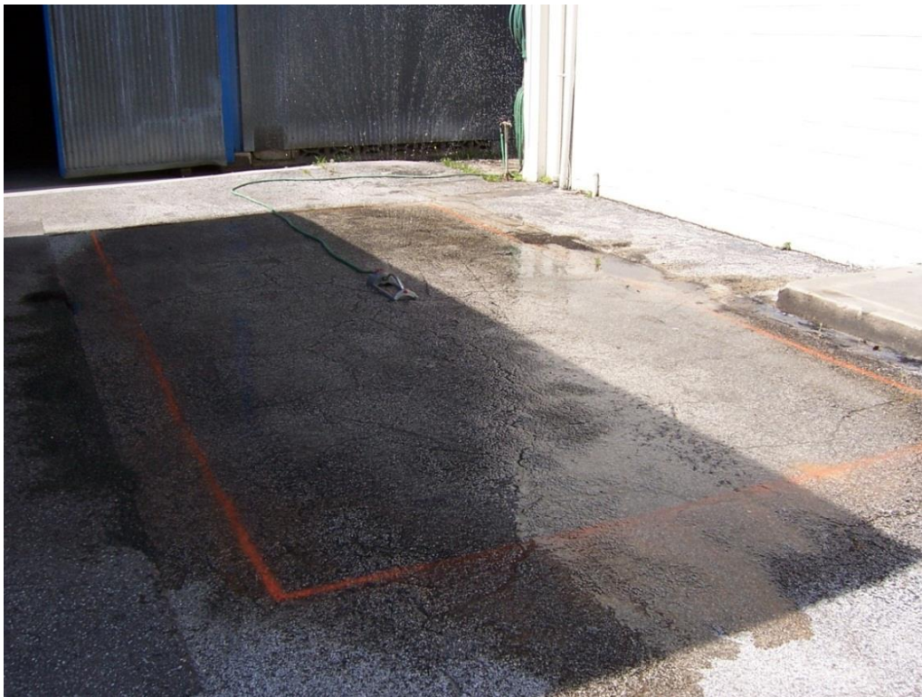
Figure 2-18. Adjusted water pressure to enclose Soil Box footprint.
