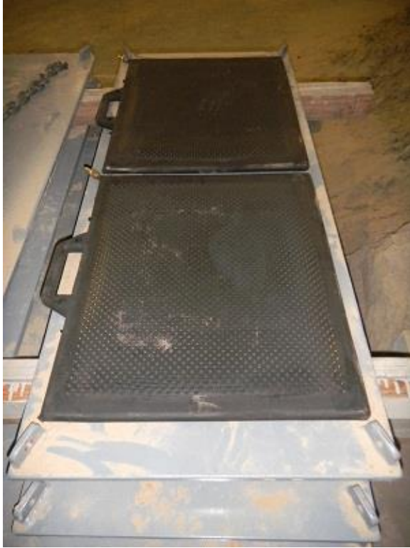
Figure 4-6. Addition of one small lift bag to small load plate.
