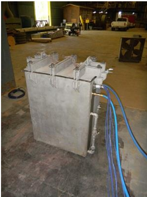
Figure 4-5. Pressure vessel checking factory calibration of pressure cells.
