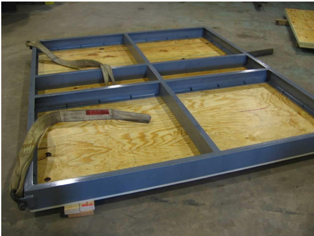
Figure 8-2. Trench box wall with first side of plywood.
