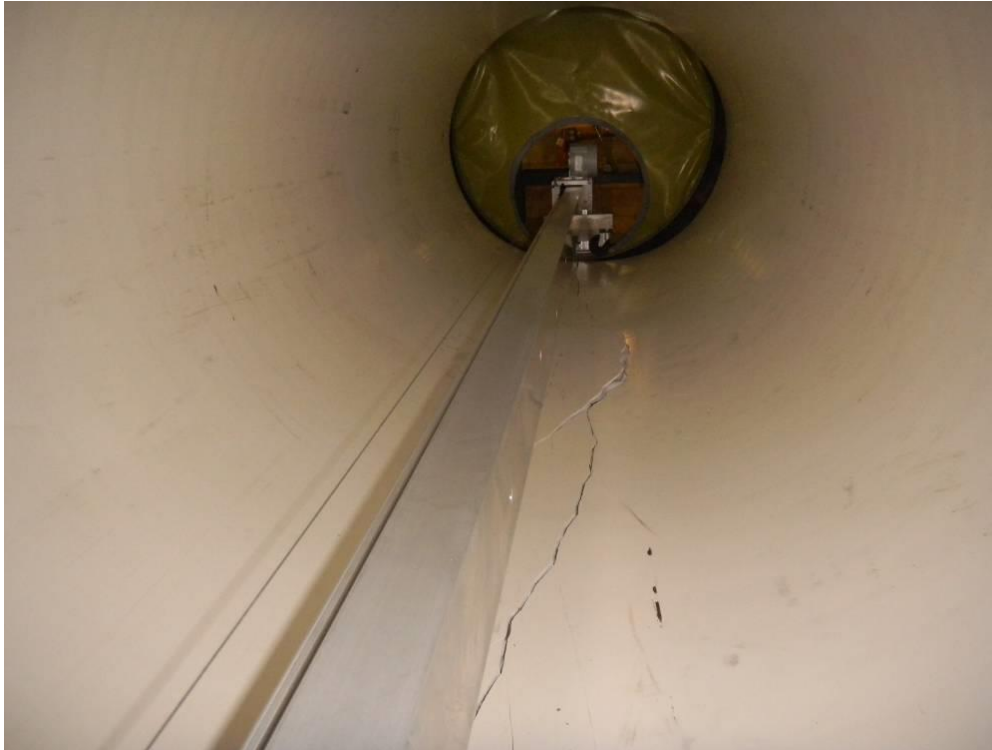
Figure 6-8. South pipe failure.
