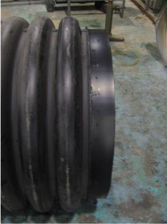
Figure 8-5. HDPE pipe end modification.
