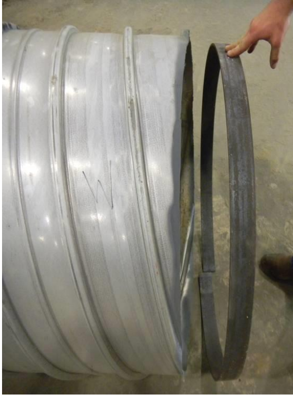
Figure 7-1. Before steel pipe end modification.
