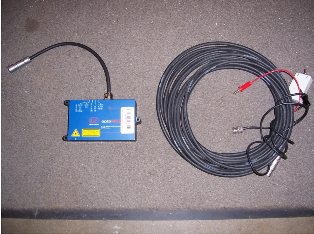
Figure 2-12. Displacement laser and cabling.
