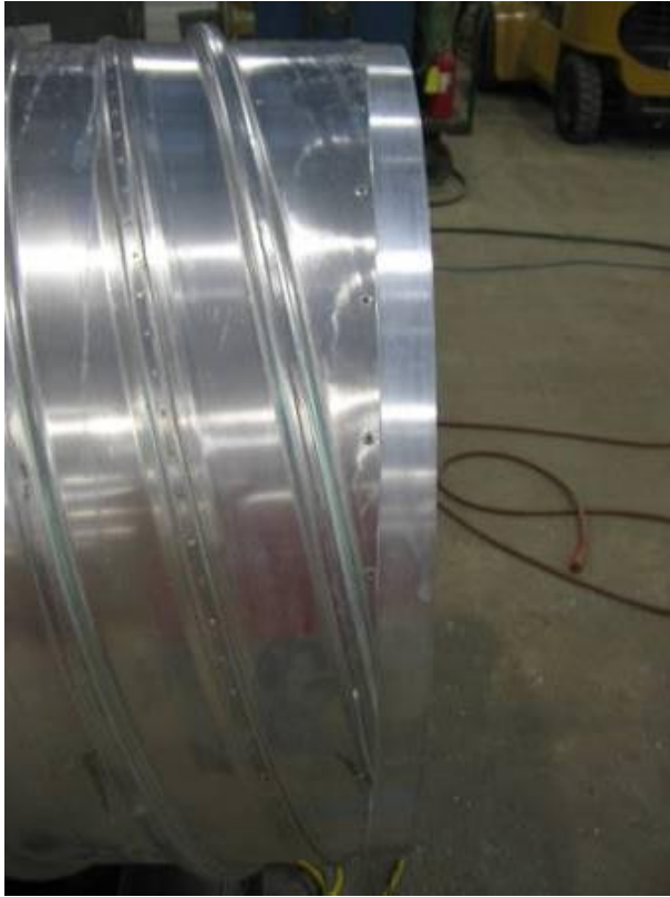
Figure 9-1. Aluminum pipe end modification
