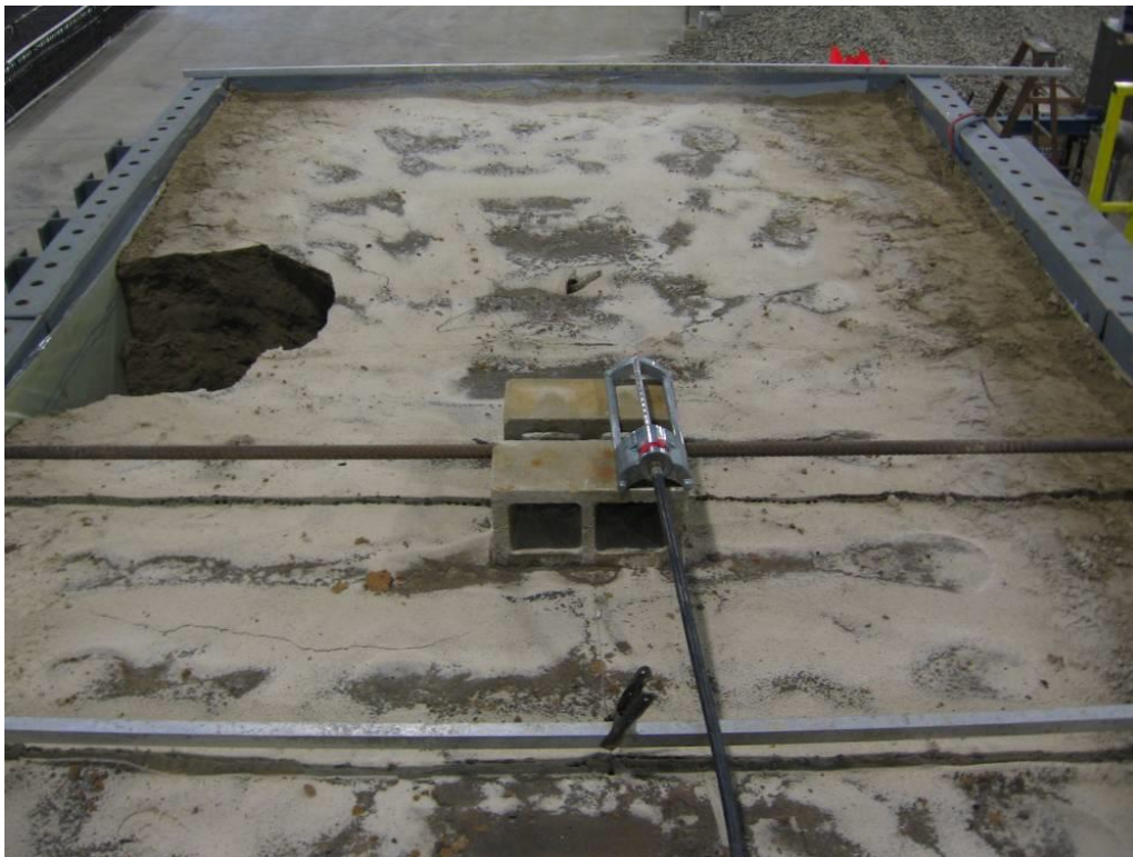
Figure 8-21. Void formed from flexible membrane breach.
