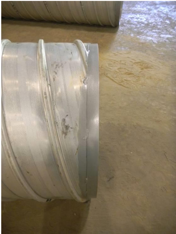
Figure 8-4. Steel pipe end modification.
