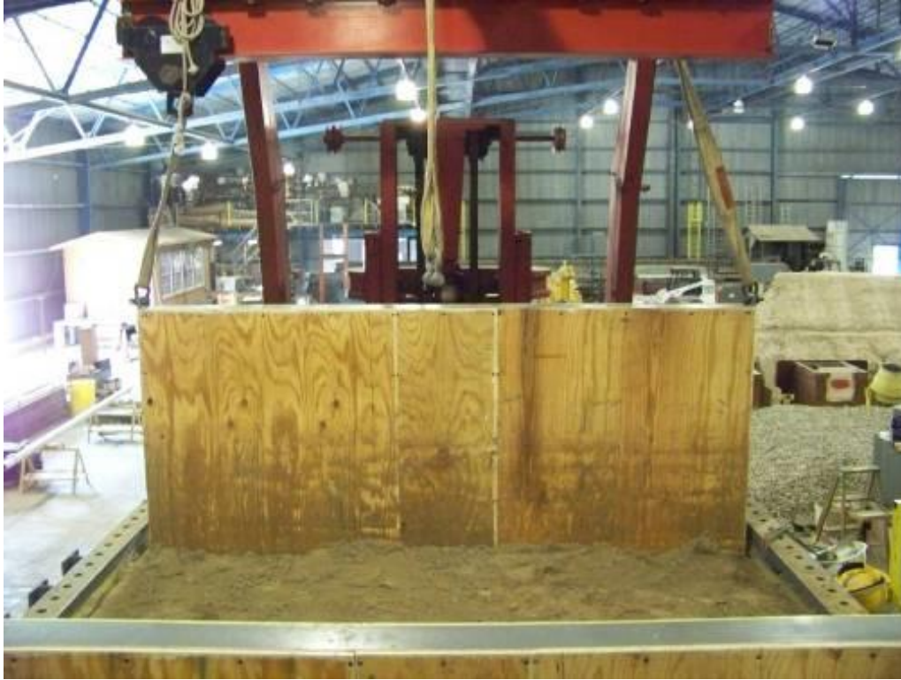
Figure 8-9. Trench box removal
