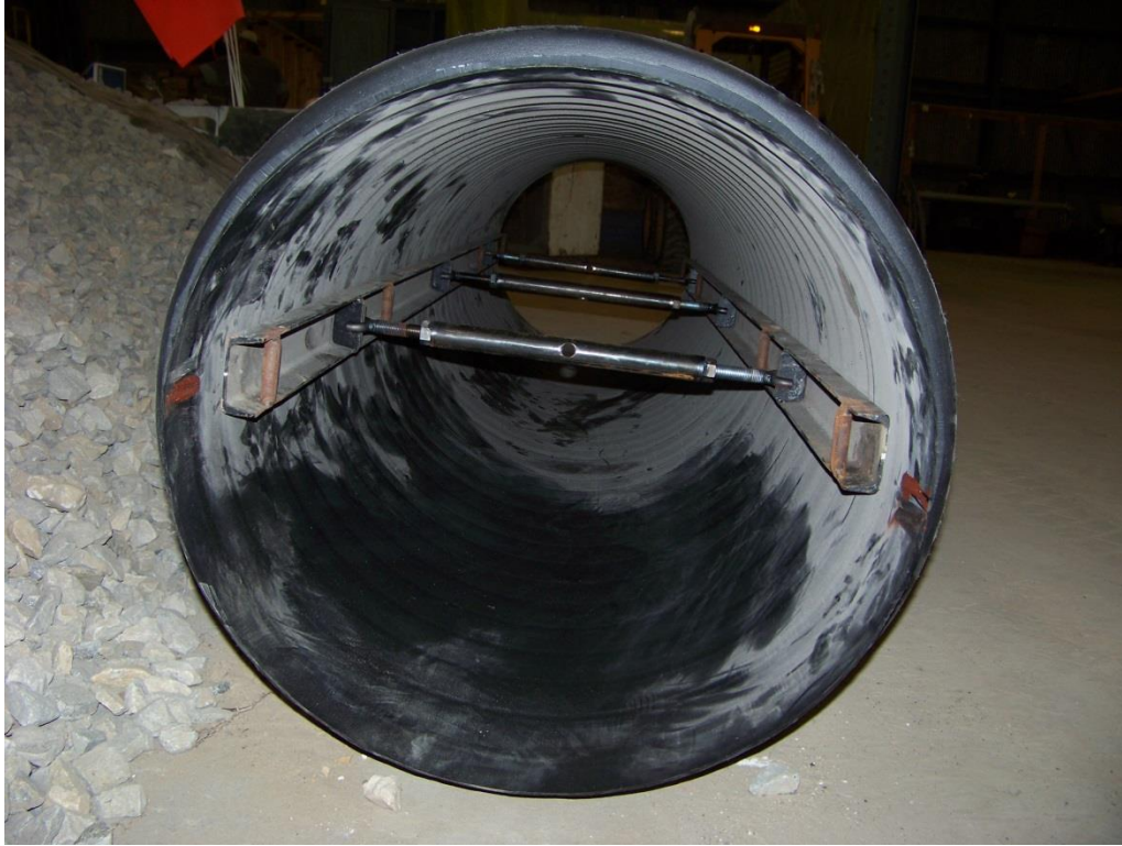
Figure 5-1. Example pipe pre-deflected to 4% of its nominal diameter.
