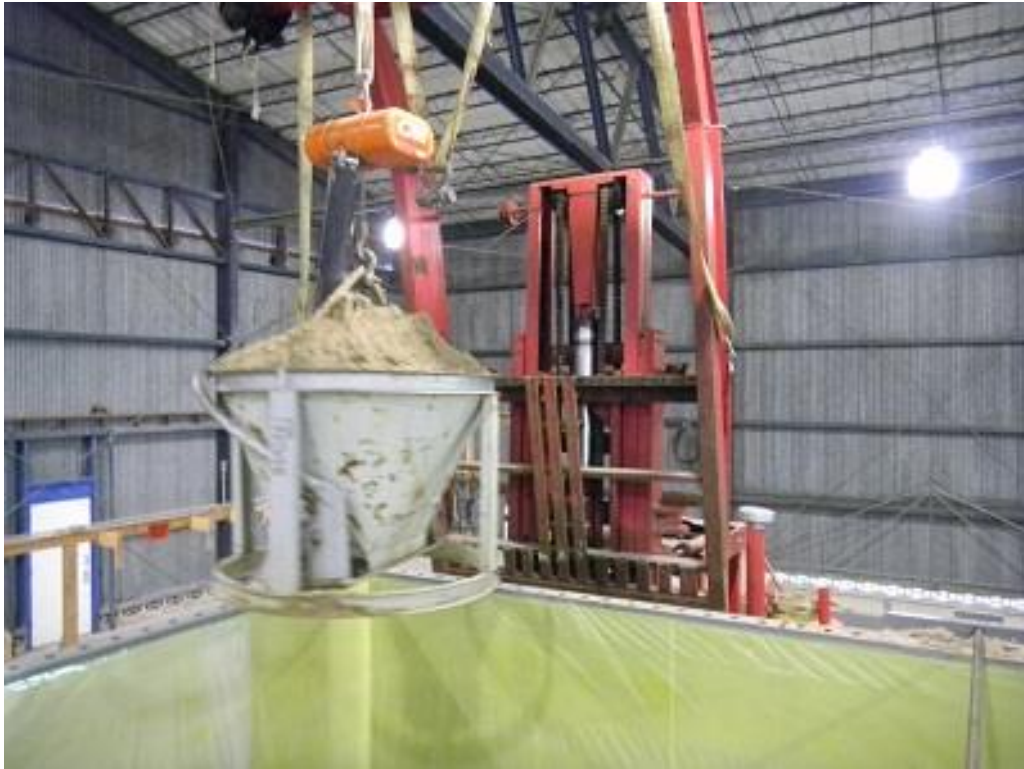
Figure 5-11. Soil being hoisted into Soil Box.
