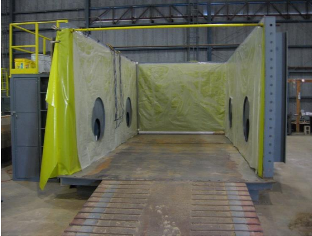
Figure 5-3. Installed lubricated polyethylene sheets.
