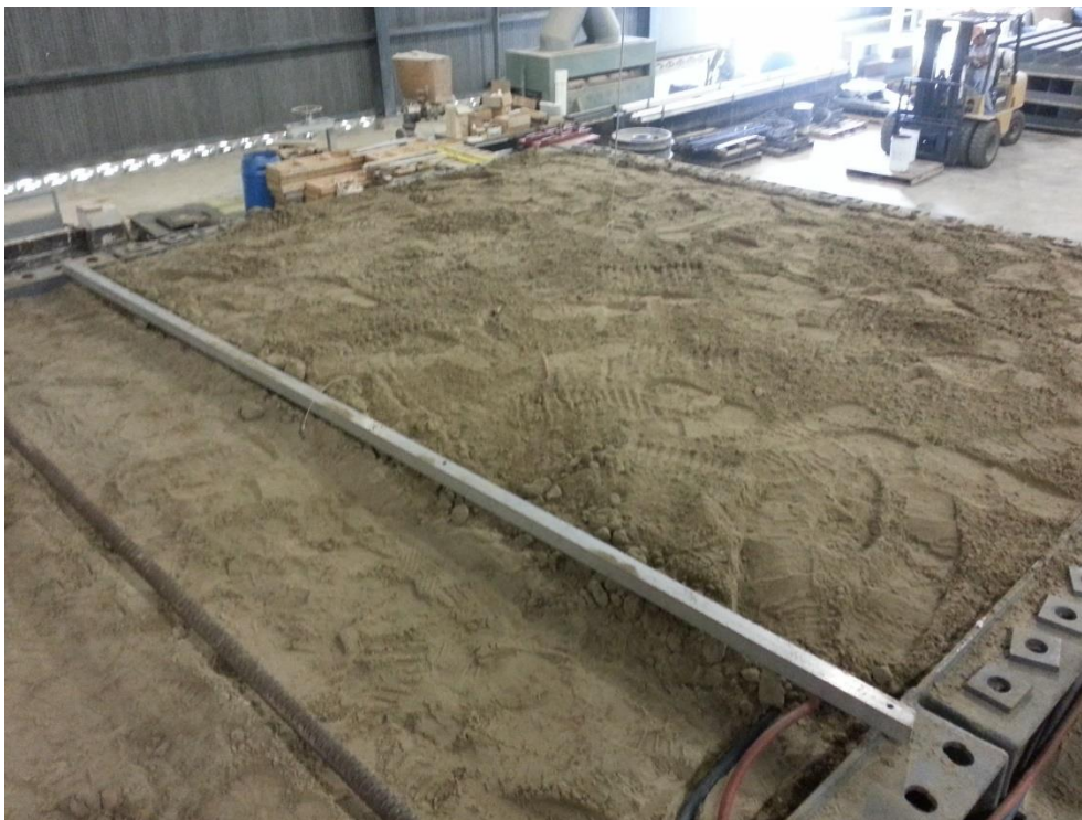
Figure 11-14. Photograph of new testing technique showing fully-buried lift bags
