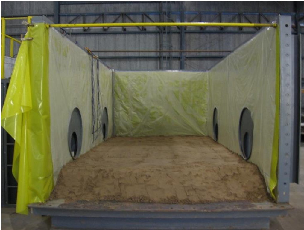
Figure 5-6. First lift after compaction.
