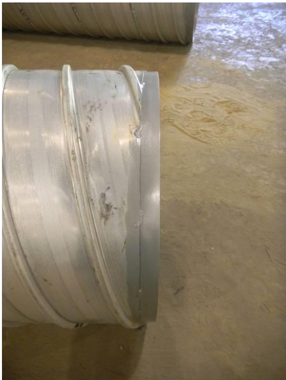
Figure 7-2. After steel pipe end modification.
