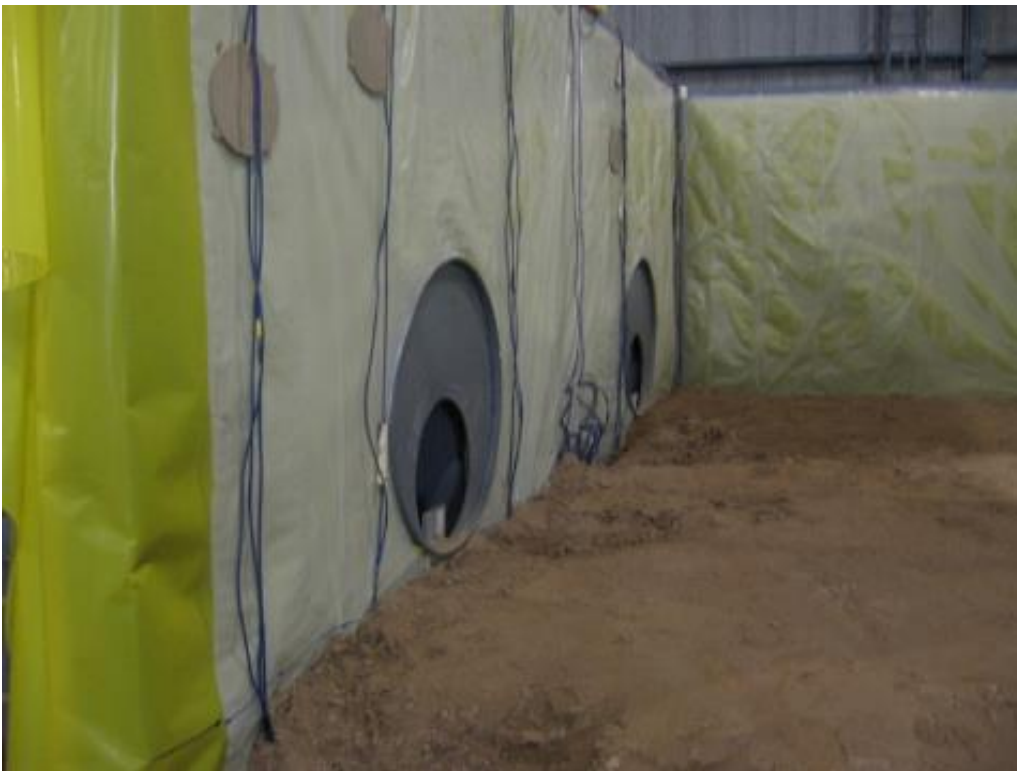
Figure 8-6. Rerouted pressure cell cabling.
