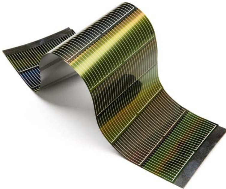
Figure 2.8 Thin film PV module: Copper Indium Gallium di-Selenide (CIGS - \text{CuInGeSe}_2 ) type (Courtesy: http://www.greentechmedia.com/wp-content/uploads/2009/02/tf-global-solar.jpg )
