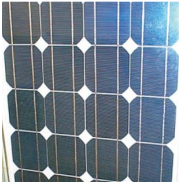
Figure 2.6 Bulk type mono-crystalline PV module (Courtesy: http://www.lowcarboneconomy.com/Resources/UserImages/gb-sol-photovoltaic2320x320.jpg )
