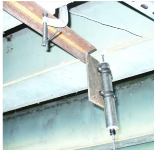
Figure 29 – Deflection gage on steel girder
