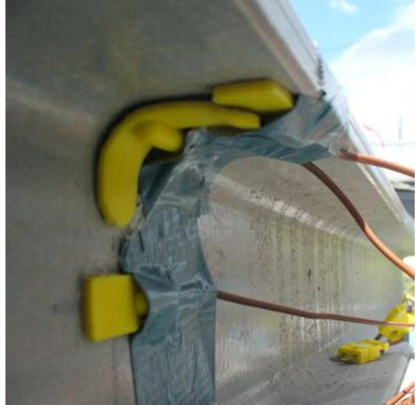
Figure 27 – Surface-temperature-measuring thermocouples on panel B8
