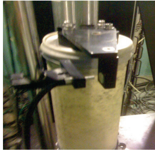
Figure 3-5. Controlling units of fixed-free RC equipment: (a) resonant column interface unit and servo amplifier unit, (b) pressure control panel, and (c) fiber optic sensor placed facing the target attached to specimen.
