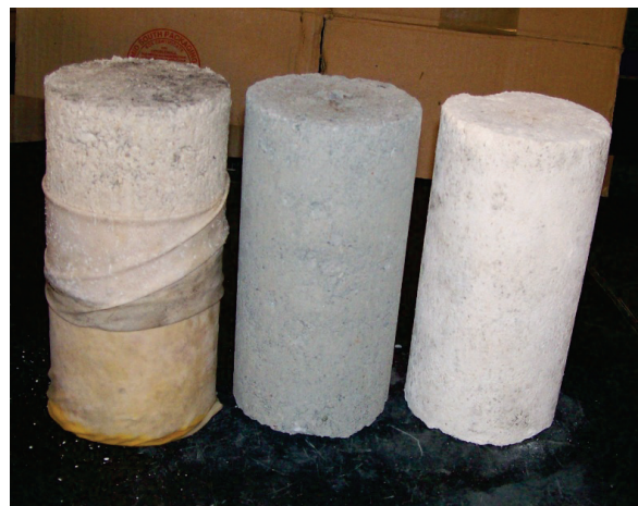
Figure 4-4. Wet specimen compaction: (a ) modified Proctor compactor with 4 inch diameter and 8 inch height specimen mold, (b) soaked aggregate trays with nylon cover sheet, and (c) compacted wet specimens of 4 inch diameter and 8 inch height.
