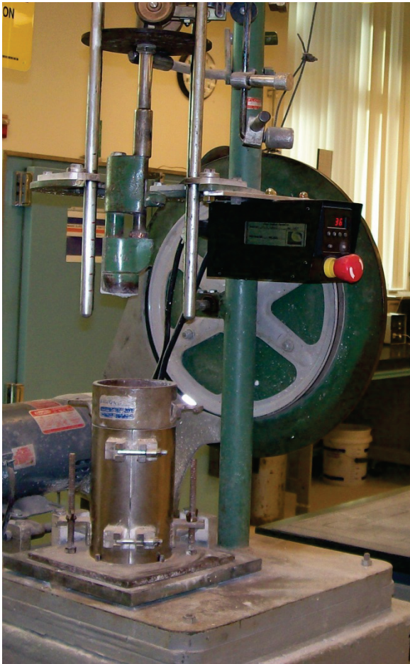
Figure 4-4. Wet specimen compaction: (a ) modified Proctor compactor with 4 inch diameter and 8 inch height specimen mold, (b) soaked aggregate trays with nylon cover sheet, and (c) compacted wet specimens of 4 inch diameter and 8 inch height.
