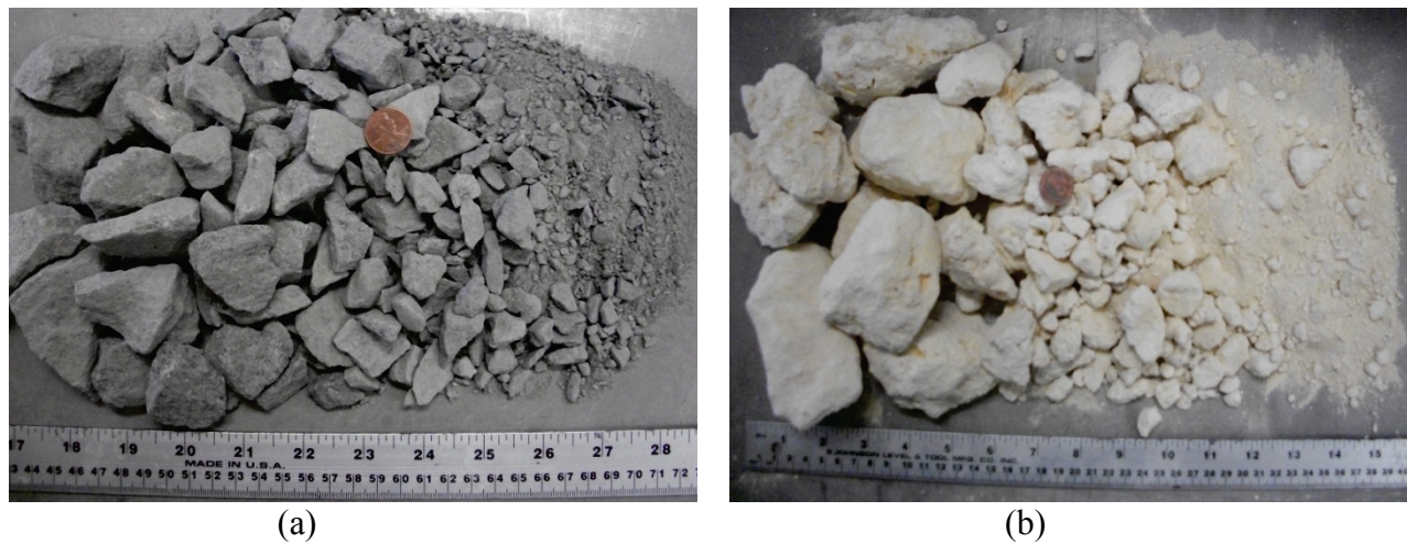
Figure 4-1. Representative samples of (a) Georgia granite and (b) Newberry limeroak.
