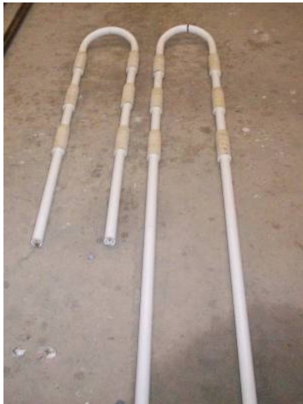
Figure 4-4 Grout delivery pipes.
