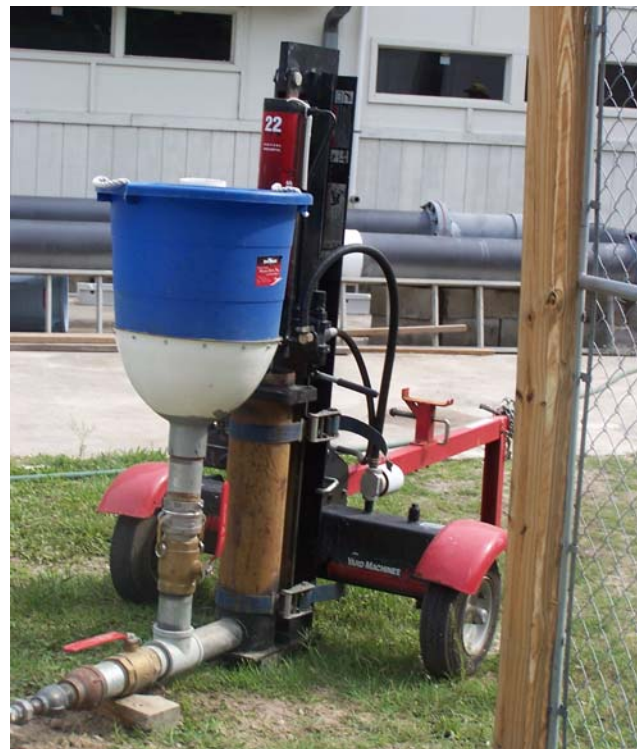
Figure 4-21 Grout pump with holding tank.
