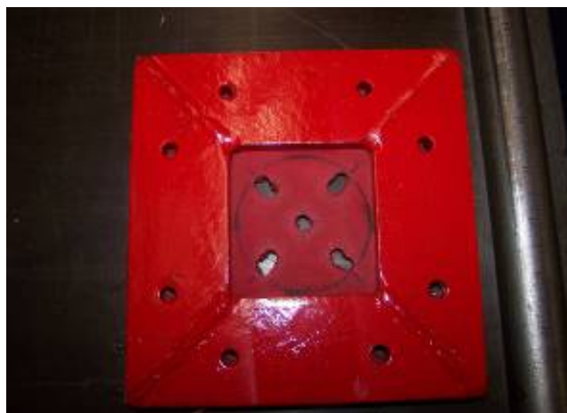
Figure 4-8 Rubber nozzle used for jetting and tip grouting.
