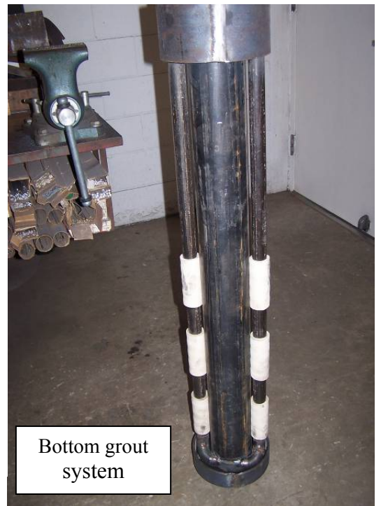
Figure 4-58 Pile with grout delivery systems.
