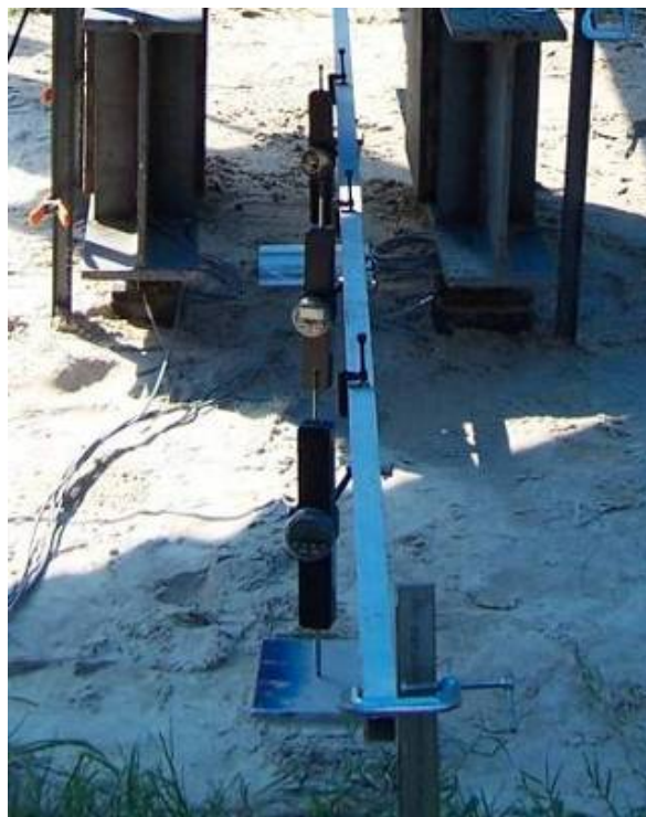
Figure 4-27 Digital dial gages for soil deformation monitoring.
