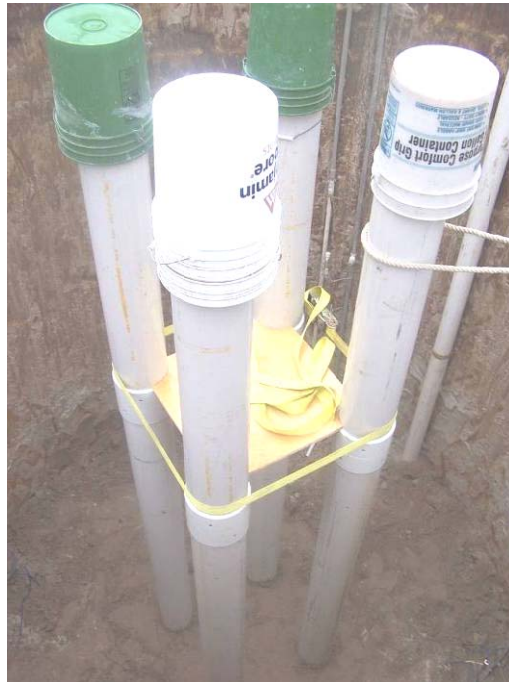
Figure 5-36 PVC casing positioned in the test chamber.
