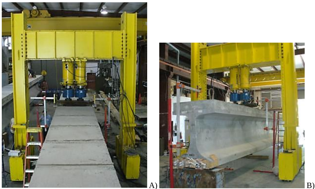
Figure 21–Test specimen and load frame view of A) top and B) side of girder
