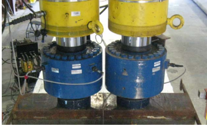
Figure 43–Load cells below hydraulic actuators
