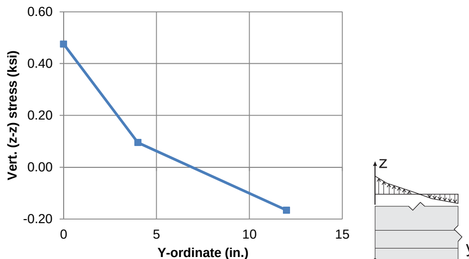
Figure 55—Estimated stress profile in web of specimen PT after transfer (tension positive)
