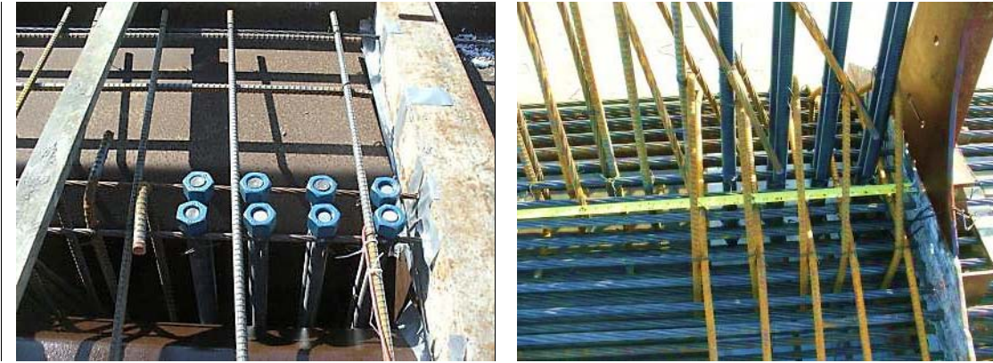
Figure 19–Top (left) and bottom (right) of all-thread rods in specimen LB
