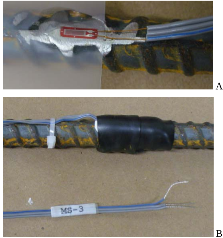
Figure 34—MS gage installation showing A) gage before protective covering and B) protective cover and label
