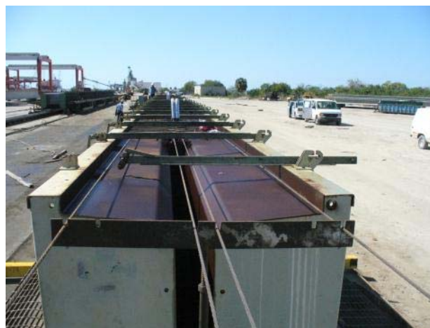
Figure 21–Form release application (left) and form cross-ties (right)
