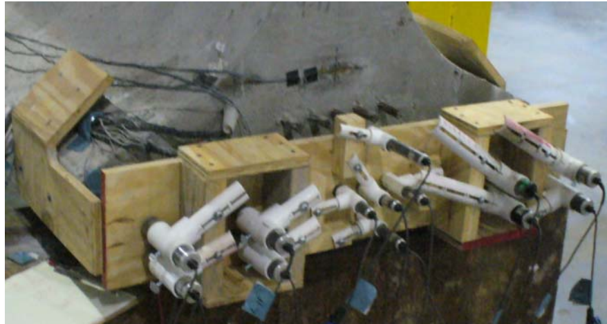
Figure 47–Wood frame and LVDTs
