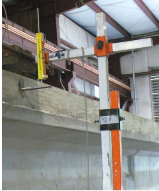
Figure 45–LVDT and support frame
