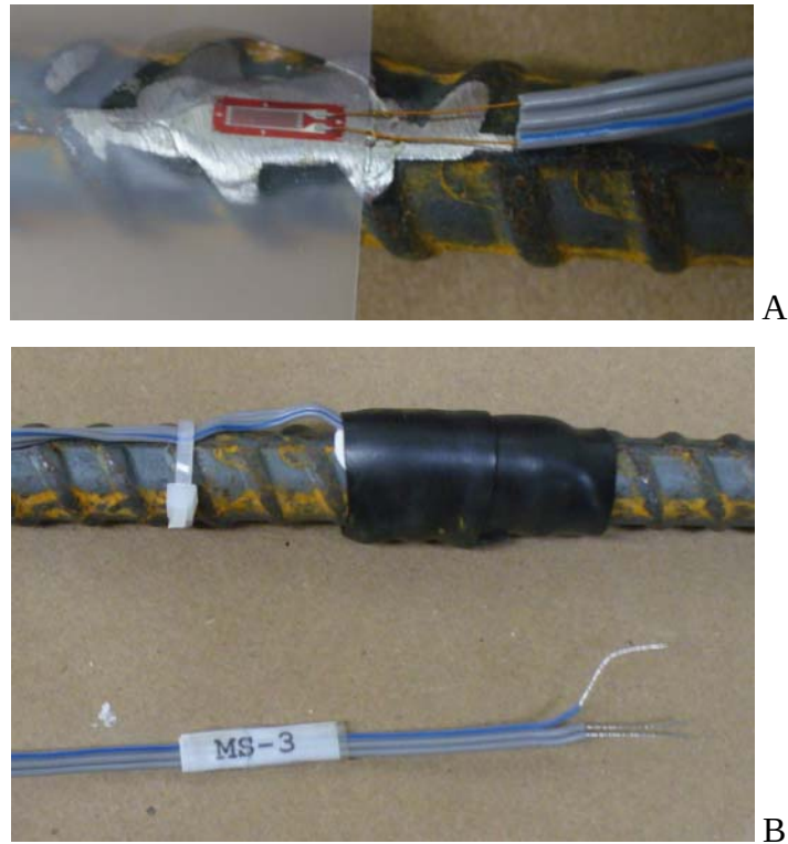
Figure 38—MS gage A) before protective covering and B) with protective cover and label
