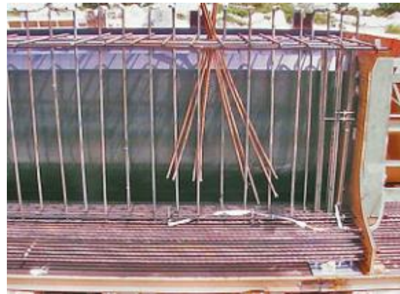
Figure 20–Girder V reinforcement A) Specimen VC and B) Specimen VU
