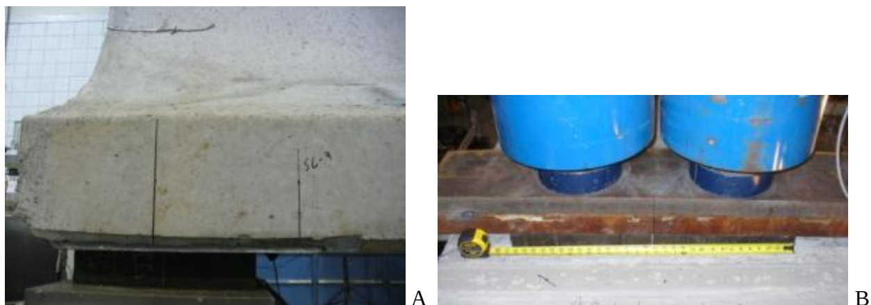
Figure 35–Test setup at A) bearing and B) load point
