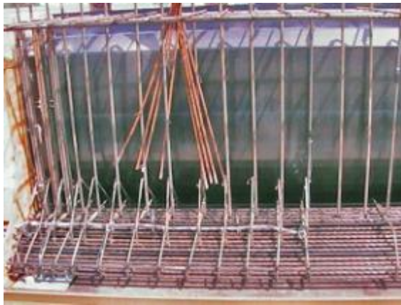
Figure 20–Girder V reinforcement A) Specimen VC and B) Specimen VU
