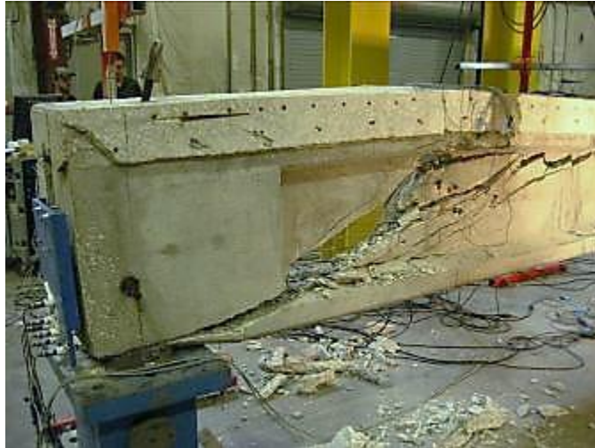
Figure 29–I2A incline cracks in web
