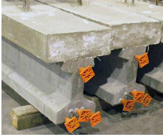
Figure 7—Finished beam specimens ready for testing
