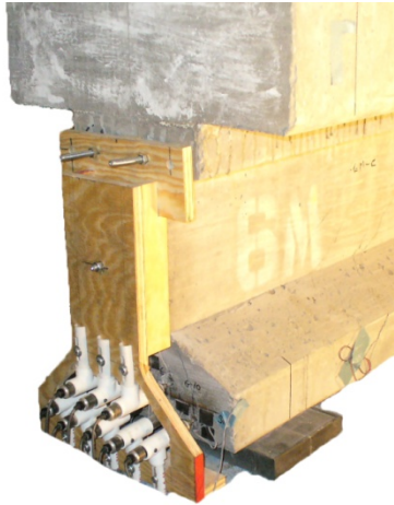
Figure 14–LVDT frame at end of beam
