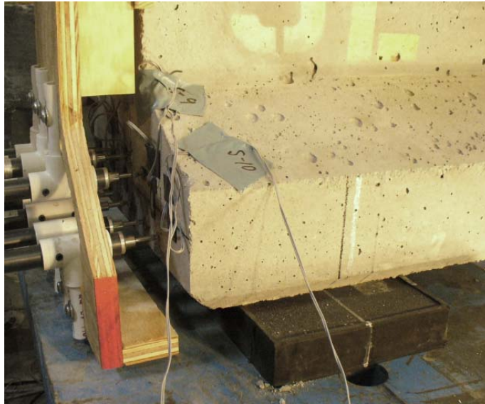
Figure 10—Specimen on bearing pad
