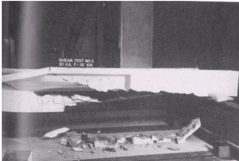
Figure 22–T-beam failure after tied-arch behavior
