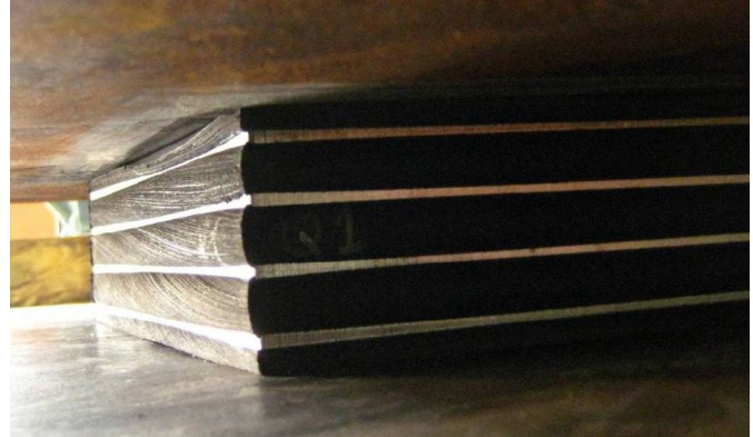
This neoprene bearing pad, in place for experimental testing, has been cut away to reveal its alternating layers of neoprene and steel.
