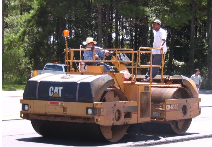
Figure 4-10. Caterpillar CB-643C vibratory roller used for dynamic compaction
