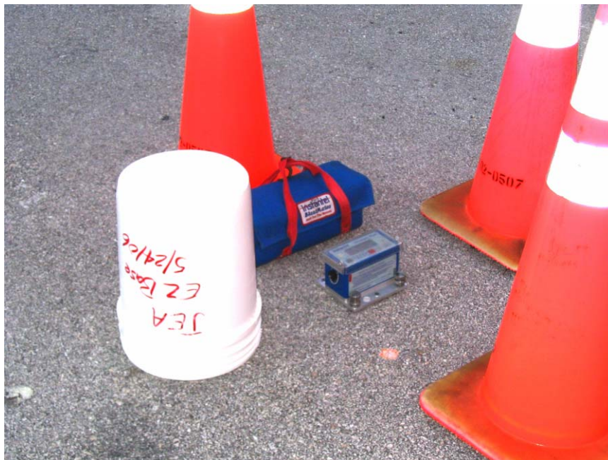
Figure 4-8. Typical vibration monitor with protective cones (bucket removed)
