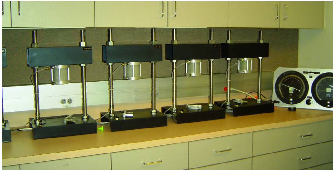
Figure 3.1 Set of PLD's, pneumatic loading device
