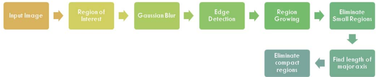
Figure 15: Flow diagram of the algorithmic steps to detect cracks in rails.
