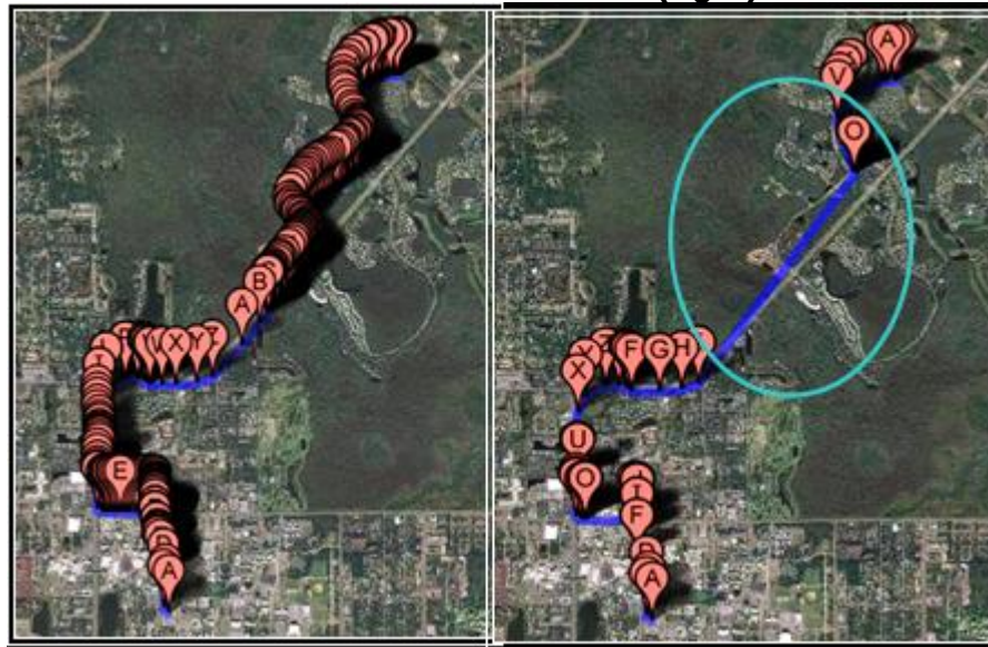
Figure 21 - Car Trip with all GPS Points (left) vs. Critical Points (right)
