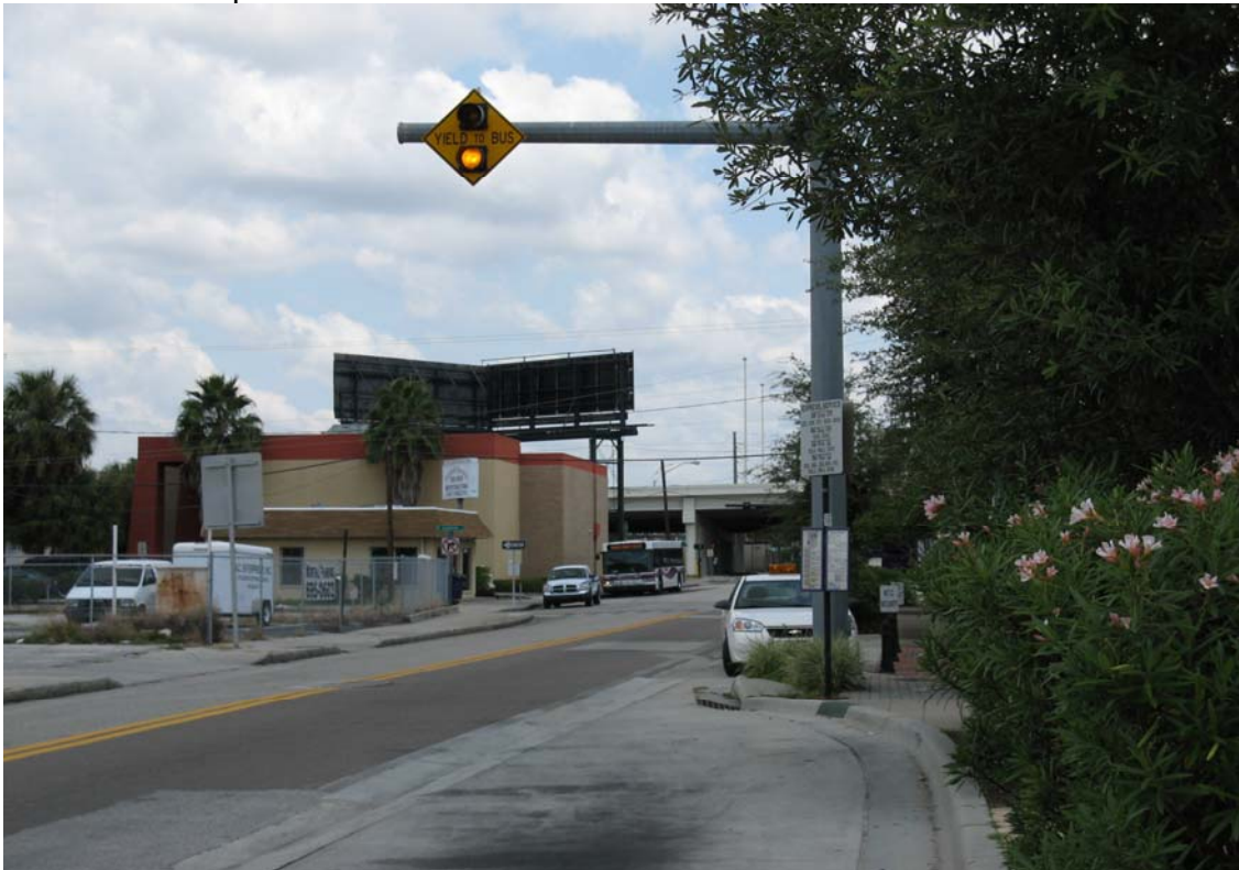
Figure 51 Yield-to-Bus Roadway Flashing Beacons
