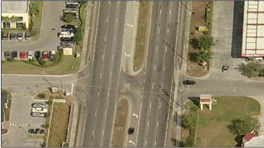
Figure 3-5: A 2x6 Four-Legged Unsignalized Intersection with an Open Median
