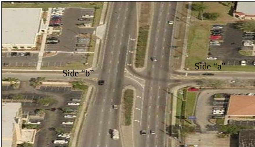
Figure 3-3: Two 2x6 Unsignalized Intersections with a Dual Directional Median
