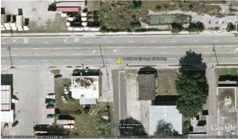
Figure 3-6: A 2x4 Three-Legged Unsignalized Intersection with a Two-Way Left Turn Lane Median
