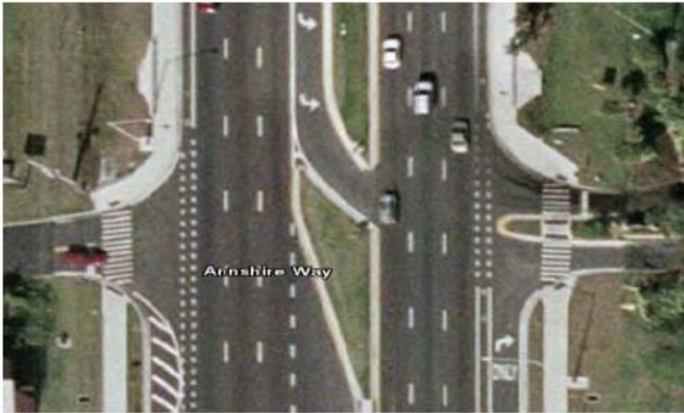
Figure 3-30: Mixed Median Type on the Major Approach (Directional from One Side, and Closed from the Other Side) to Illustrate the Idea of Having Two 3-Legged Unsignalized Intersections Facing Each Other (Having the Same Intersection Node Number, Mile Point and Roadway ID)
