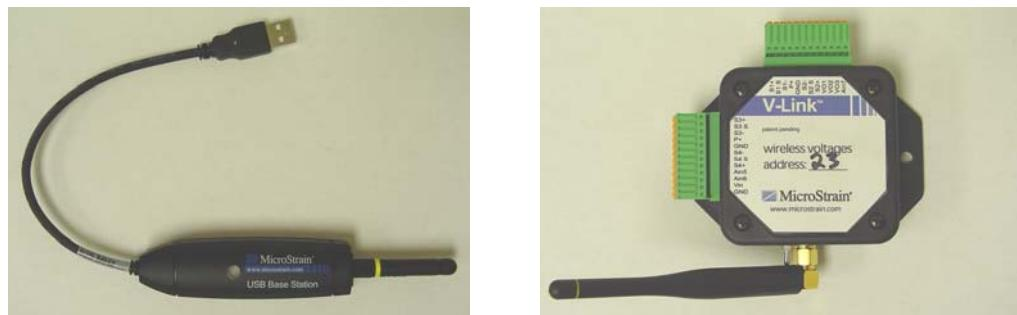
Figure A.4 – Microstrain data acquisition and transmitter
