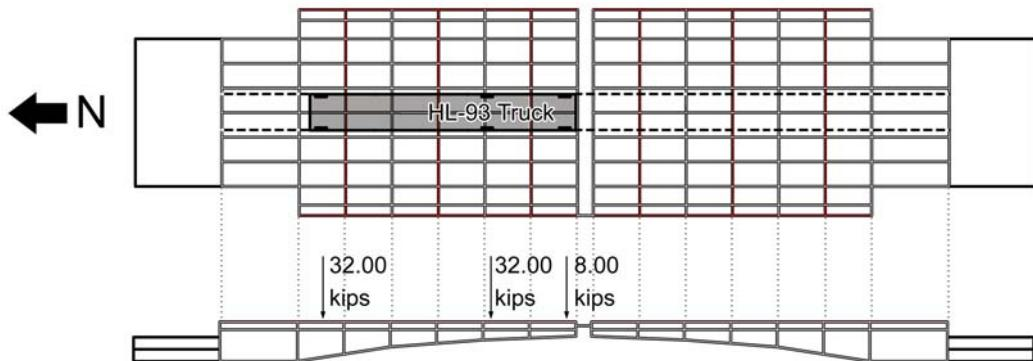
Figure 4.32 – Loading position for FEM analysis results
