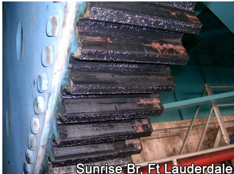
Figure 5.13 – Open gear / rack
