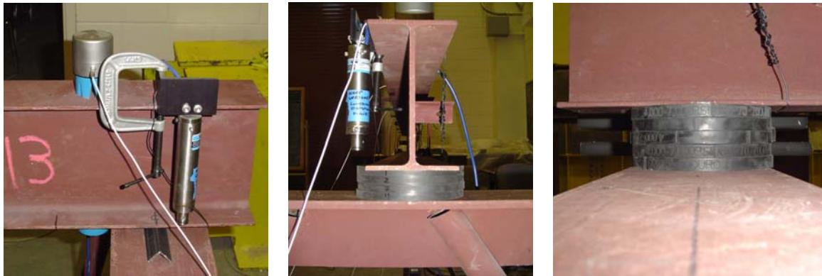
Figure B.8 – Example pictures showing different BC (a) The pin support for BC1
