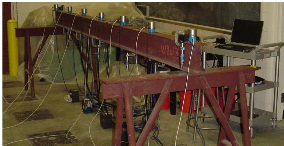
(a) Instrumented steel beam
