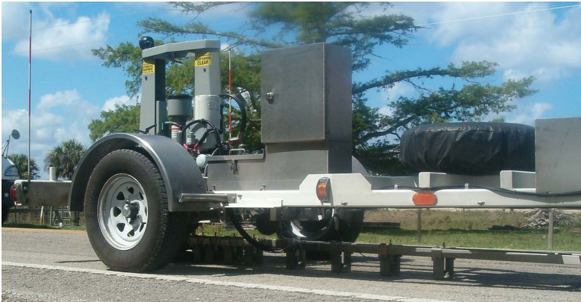
Figure 4.2: Dynatest Deflectometer with Sensor Bar Deployed During a Test
