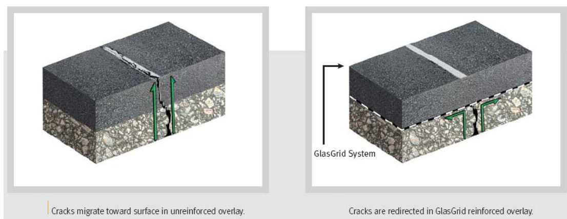
Figure 3.5: Resistance to Bottom-up Cracks (from Tensar Corp.)
