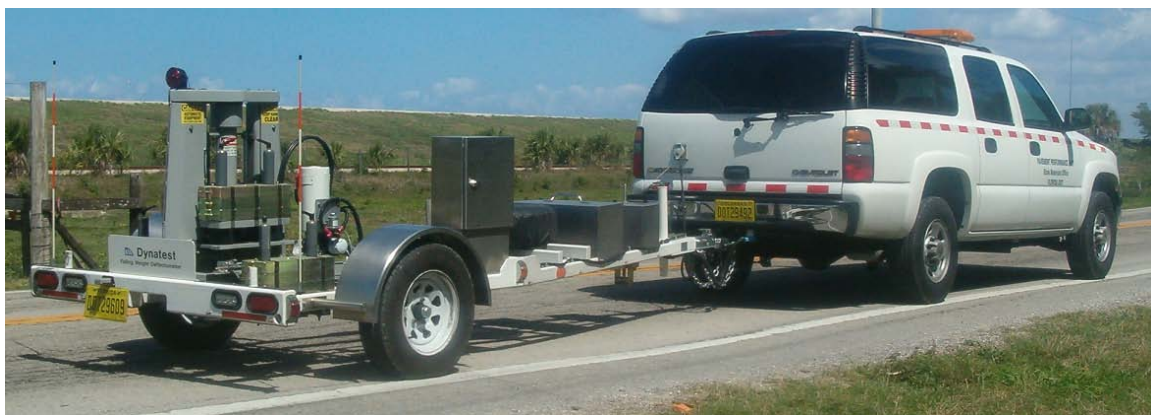
Figure 4.1: Dynatest Deflectometer and Tow Vehicle on SR15/US98
