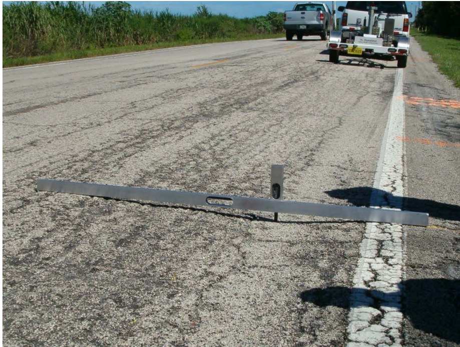
Figure 4.3: Rut Depth Measurement on SR15 / US 98
