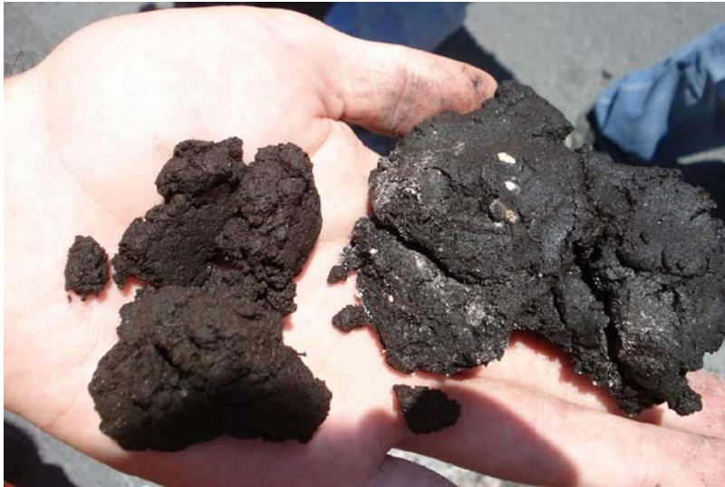
Figure 1.1: Silty “Muck” Soil Samples at SR15 Test Site
