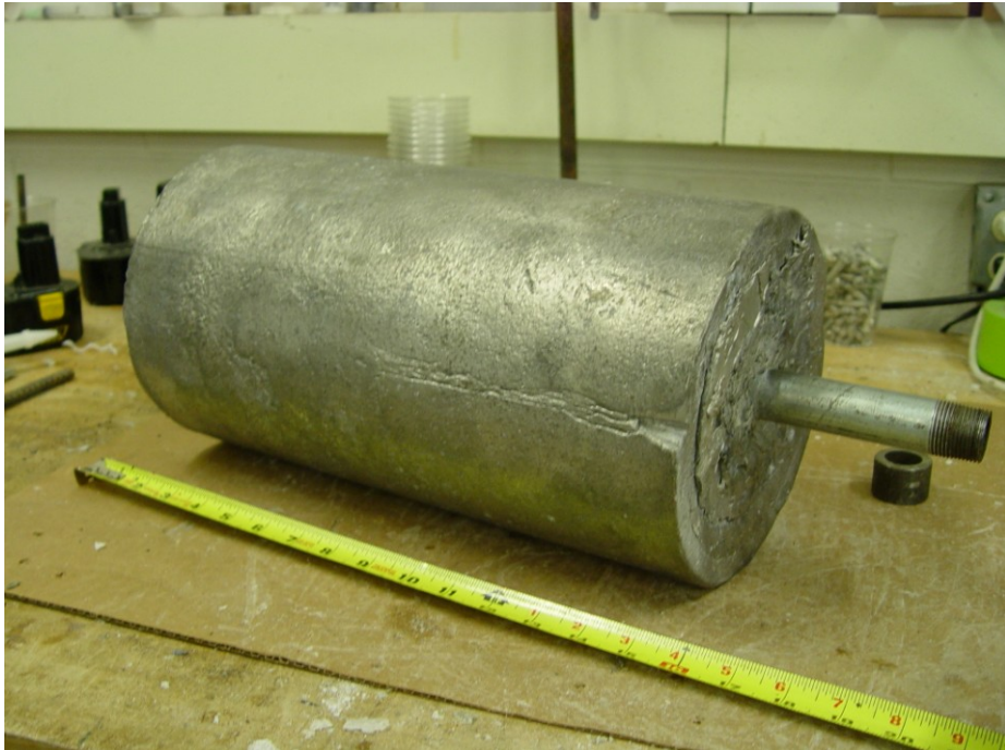
Figure 31: Photograph of a 22.6 kg pier type Mg anode as-received.
