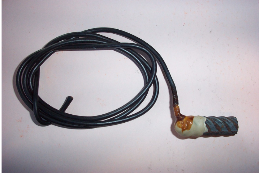
Figure 13: Photograph of a monitoring probe and connection cable prior to embedment.
