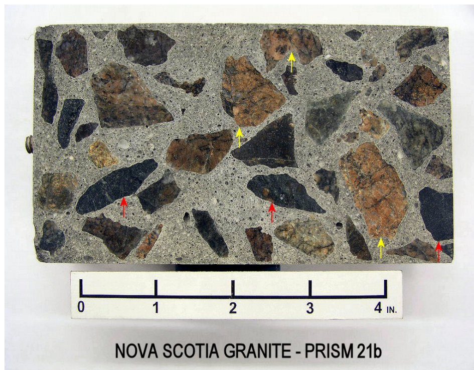
Figure VIII-32: Lapped section views of Prism 21b which contains the NG coarse aggregate. The yellow arrows point to particles referred to as light-colored particles. The red arrows point to particles referred to as dark particles.
