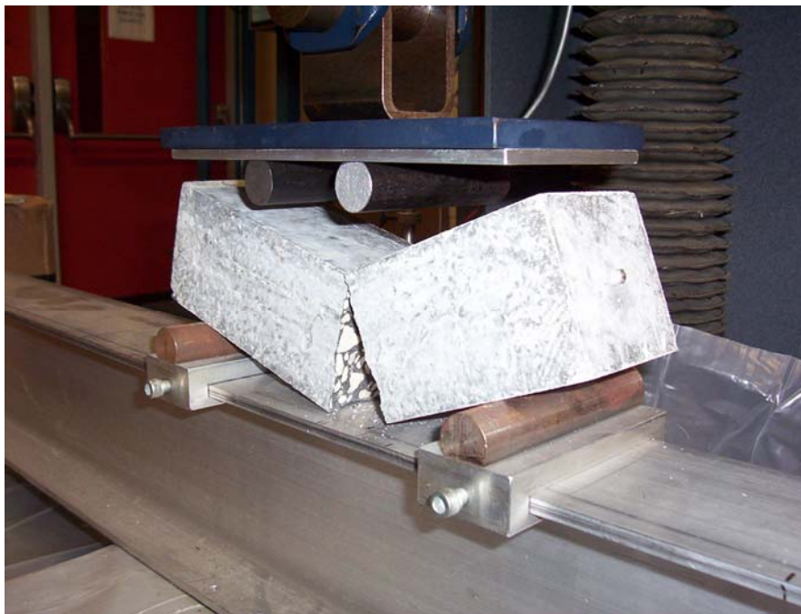
Figure VIII-47: Specimen 54b after flexural stress testing.
