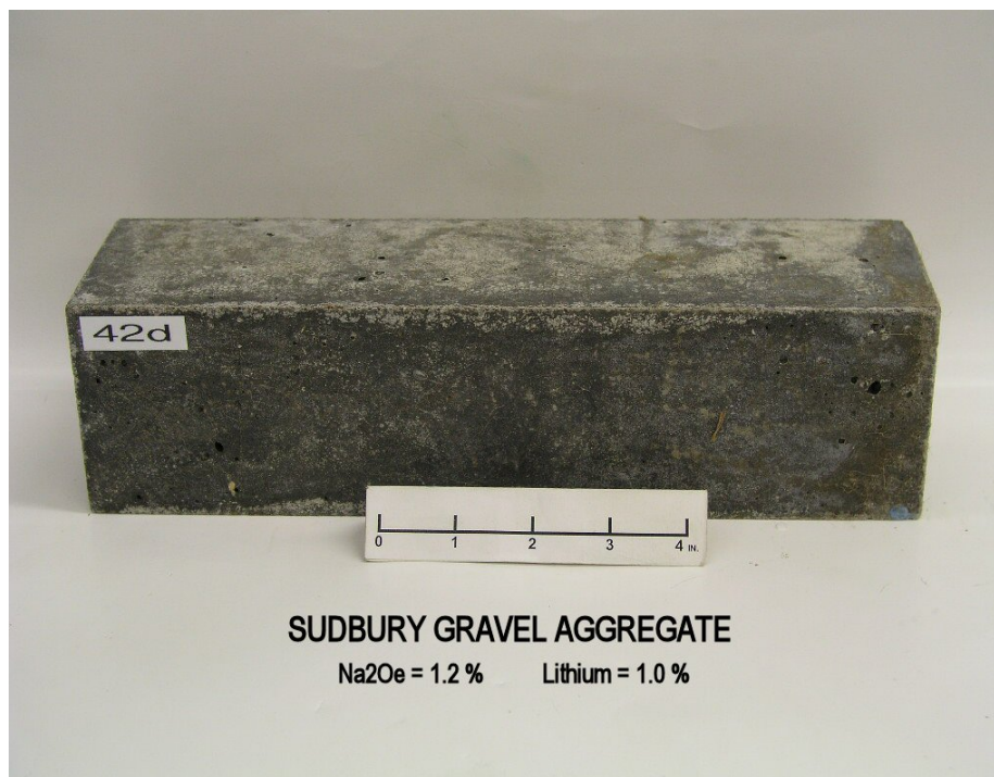
Figure VIII-41: Prisms 40d and 42d following one year exposure in the ASTM C 1293 test. At the highest alkali content of 1.2 percent, Prism 40d with no lithium admixture had an expansion of 0.0144 percent. Prism 42d, with the same alkali content and the higher lithium admixture dosage, had an expansion of 0.0069 percent. Neither prism showed any cracking at one year.
