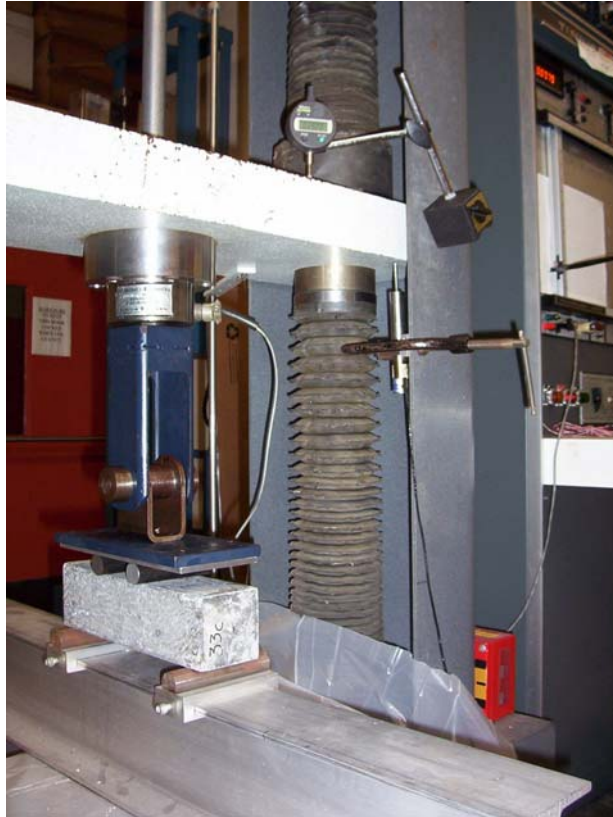
Figure VII-6: Photograph of the experimental setup for flexural strength tests.
