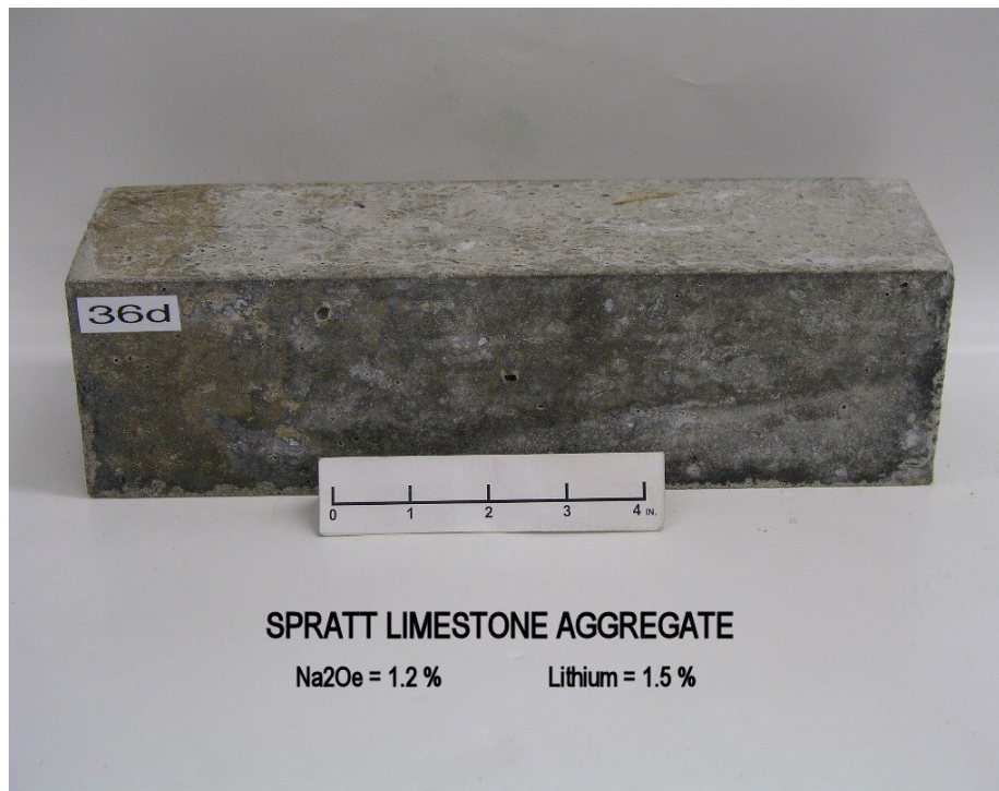
Figure VIII-39: Prisms 32d and 36d following one year exposure in the ASTM C 1293 test. At the highest alkali content (1.2 percent) Prism 32d with no lithium admixture had an expansion of 0.0796 percent. Prism 36d, with the same alkali content and the higher lithium admixture dosage had an expansion of 0.0142 percent. Only Prism 32d shows cracking (arrows).
