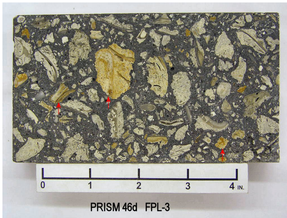
Figure VIII-25: Lapped section views of prism 46d. The arrows point to pale orange-colored particles. The majority of the aggregate particles in FPL-3 are white.
