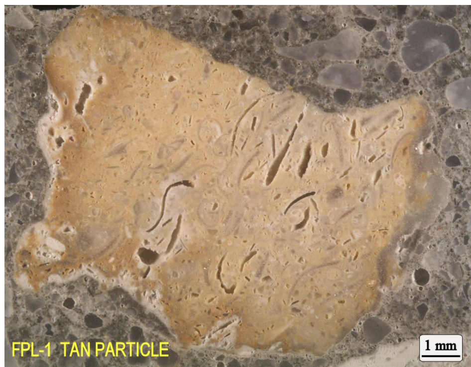
Figure VIII-15: Lapped section views of prism 9b showing enlarged views of a typical white limestone coarse aggregate particle (7X) and a typical tan limestone coarse aggregate particle (10X). The tan coloration is due in part to a clay component in some of the limestone particles. The visible porosity in the aggregate particles is primarily of the moldic variety.
