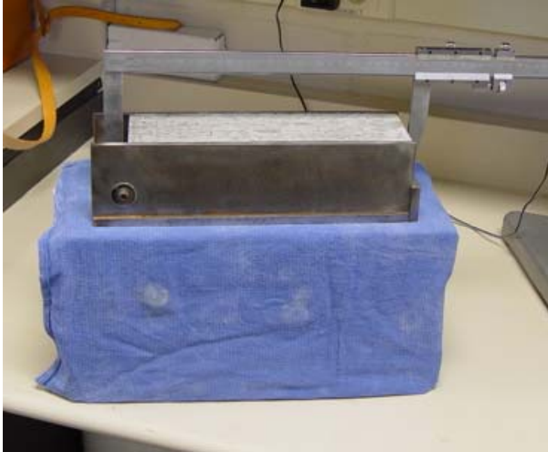
Figure VII-3: Photograph showing prism length measurement with calipers.
