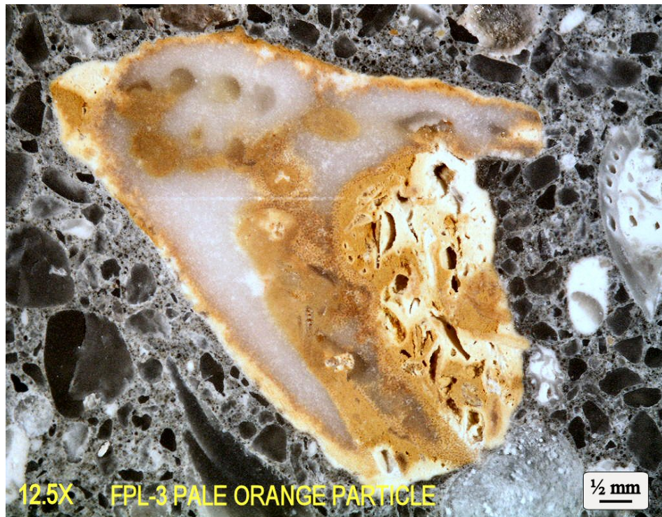
Figure VIII-27: Lapped section of prism 46d showing enlarged (7X and 12.5X) views of typical pale orange FPL-3 limestone coarse aggregate particles.
