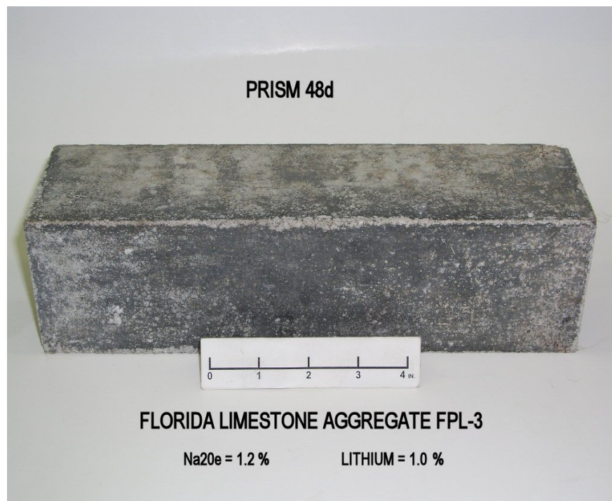
Figure VIII-28: Prisms 46d and 48d following one year of ASTM C1293 exposure. At the highest alkali content of 1.2 percent, prism 46d (no lithium admixture) had a one year expansion of 0.0089 percent. Prism 48d, with
