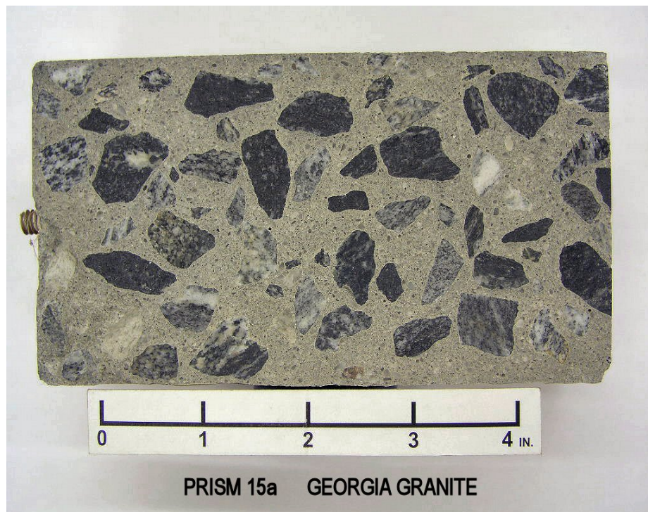
Figure VIII-29: Lapped section views of Prism 15a which contains the Georgia granite coarse aggregate. This concrete contains an alkali content of 1.2 percent and no lithium admixture.
