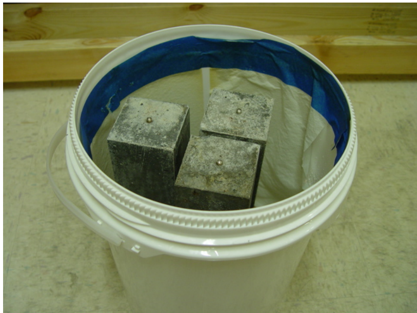
Figure VII-1: Storage container and concrete prism specimens.
