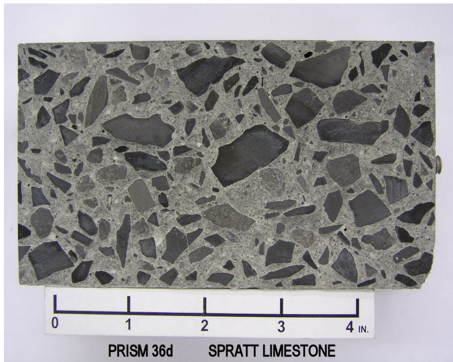
Figure VIII-37: Lapped section views of Prism 36d following one year exposure in the ASTM C 1293 test. This concrete series (36) had an alkali content of 1.2 percent and the higher lithium admixture dosage.
