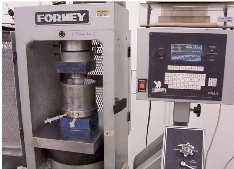
Figure VII-5: Test system for concrete pore water expression.
