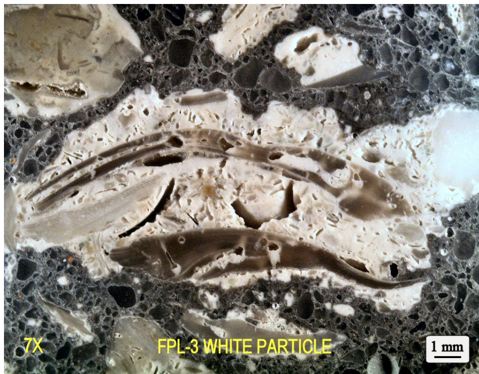
Figure VIII-26: Lapped section of prism 46d showing enlarged (7X) views of typical white FPL-3 limestone coarse aggregate particles.
