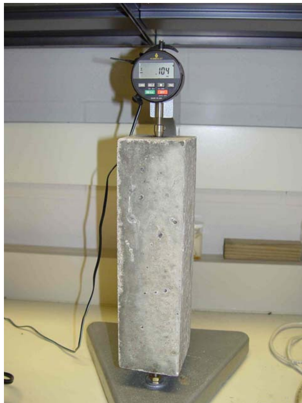
Figure VII-3: Photograph showing prism length measurement with calipers.
