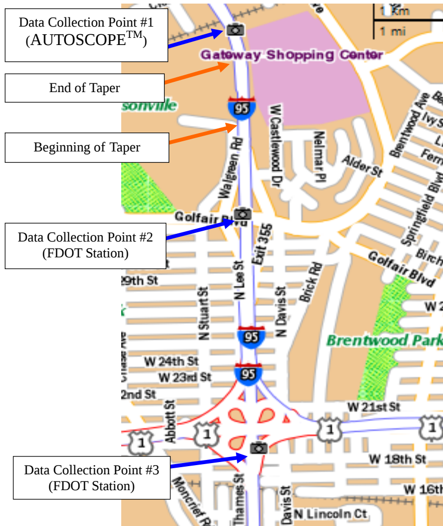
Figure 2: Data Collection Site Diagram for the Left Lane Closure
