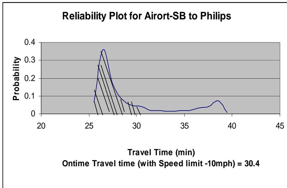
**Figure 17 Reliability Plot For O-D Pair Airport-SB To Philips (Speed Limit – 10 Mph)**
