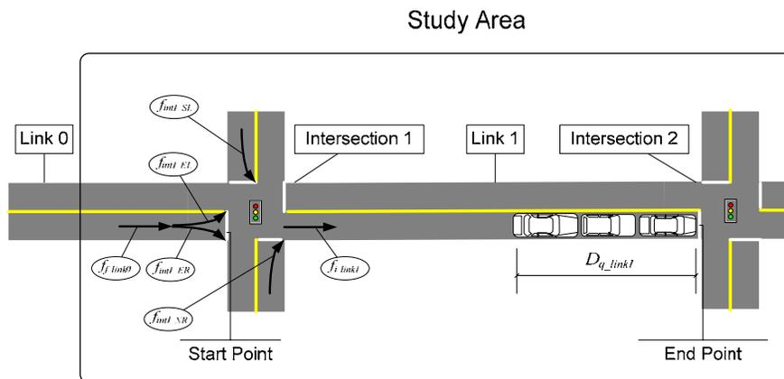
Figure 1-1: Sketch of A Link and Illustration of Significant Variables
