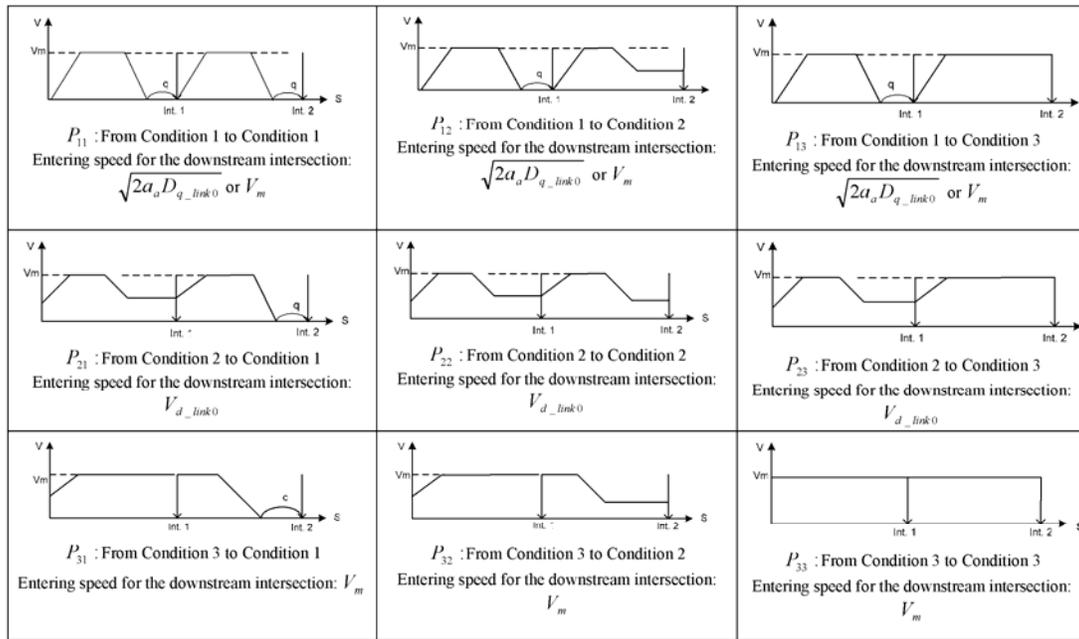
**Figure 1-2. Speed Profiles for a Vehicle Traveling Through a Link**
