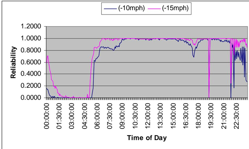
**Figure 19 Reliability Plot For Airport SB To Philips**
