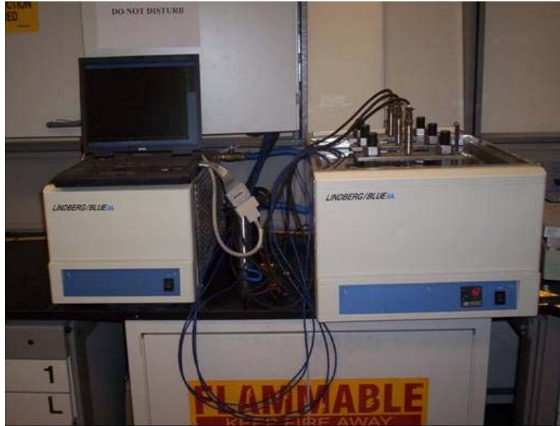
Figure 3-23. Set-up for coefficient of thermal expansion test.
