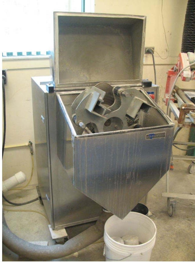
Figure 3-25. Grinder used for grinding concrete cylinder samples.
