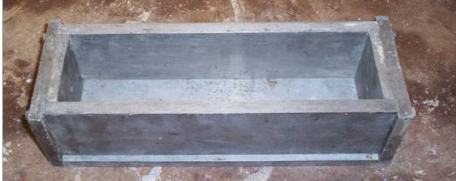
Figure 3-21. Mold for free shrinkage test.
