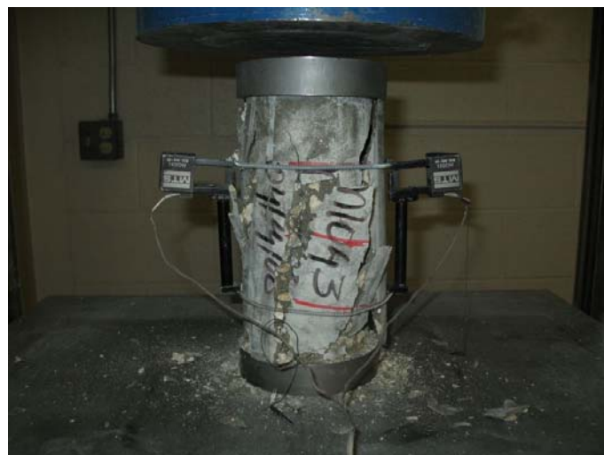
Figure 3-15. Failure of concrete cylinder in compressive strength test.
