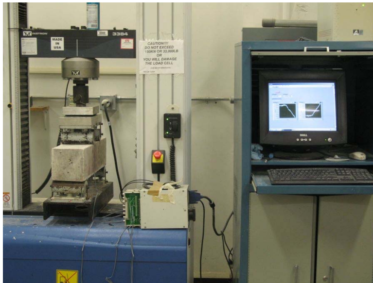
Figure 3-16. Test set-up used for flexural strength test.
