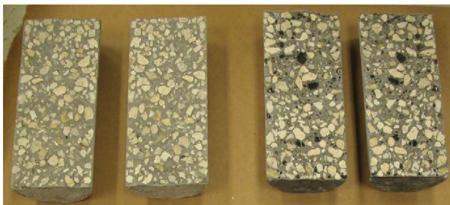
Figure 3-20. Failure of concrete cylinders in indirect tension.
