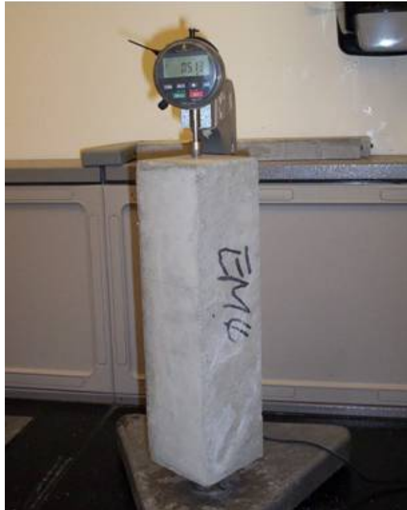
Figure 3-22. Set-up for shrinkage test.
