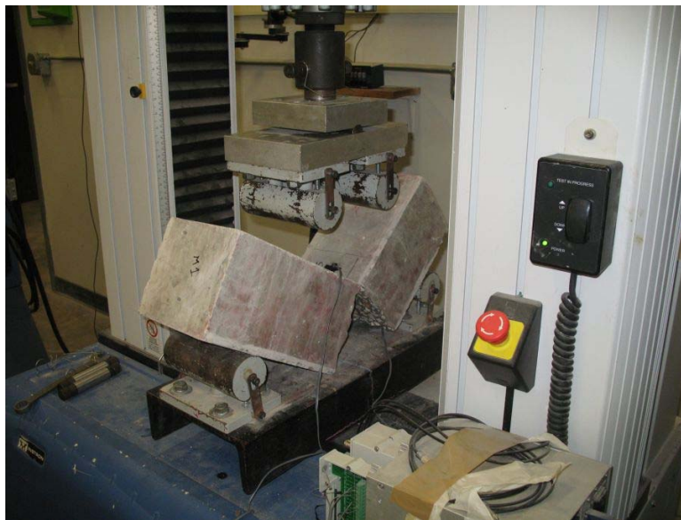
Figure 3-17. Failure of the beam without RAP material.
