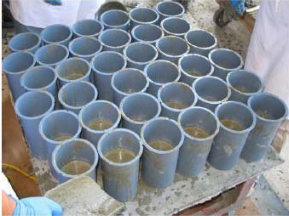
Figure 3-11. Table vibrator used to consolidate cylinder samples.
