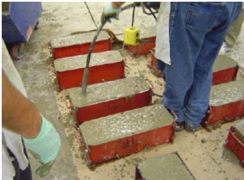
Figure 3-10. Internal vibrator used to consolidate beam samples.
