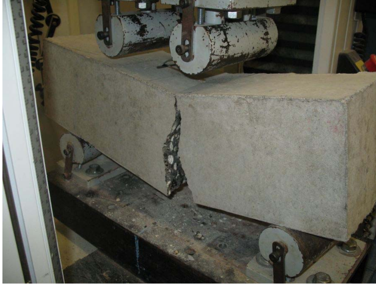
Figure 3-18. Failure of the beam containing RAP material.
