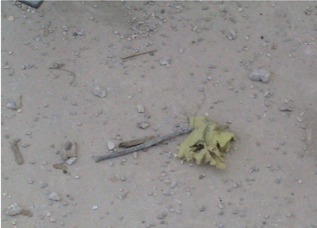
Figure 6-2. Deleterious materials from a stockpile of RCA.
