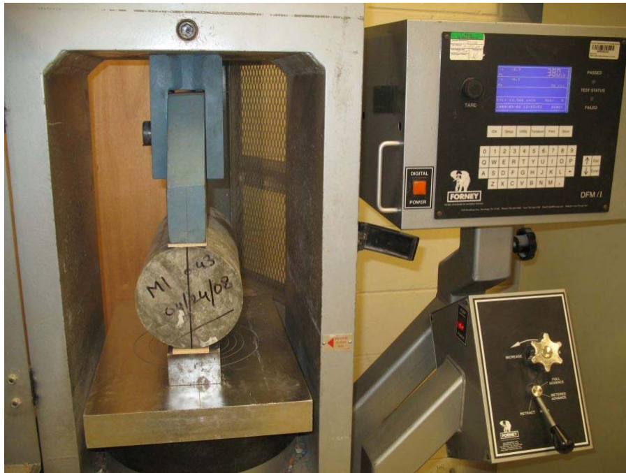
Figure 3-19. Test set-up for splitting tensile strength test.
