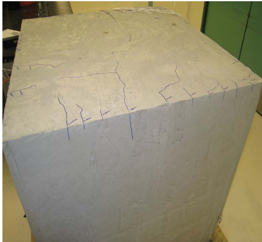
Figure 8-12. Top surface of experimental block containing Mixture 1 showing numerous cracks along the edges.
