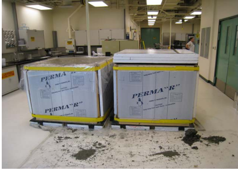
Figure 5-2. Uninsulated (left) and insulated (right) mass concrete block specimens.
