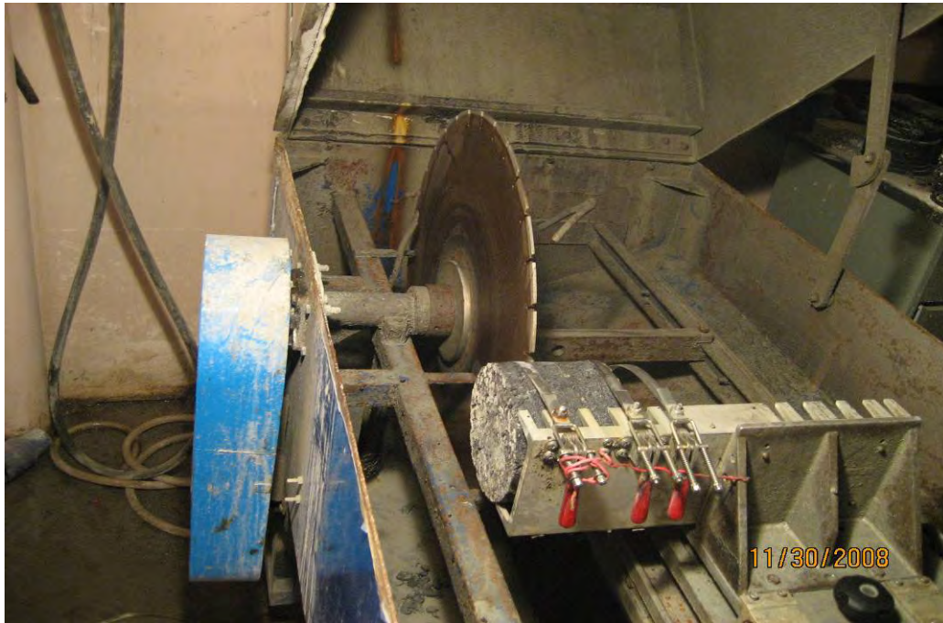
Figure 5-10 Diamond Saw Used for Specimen Slicing
