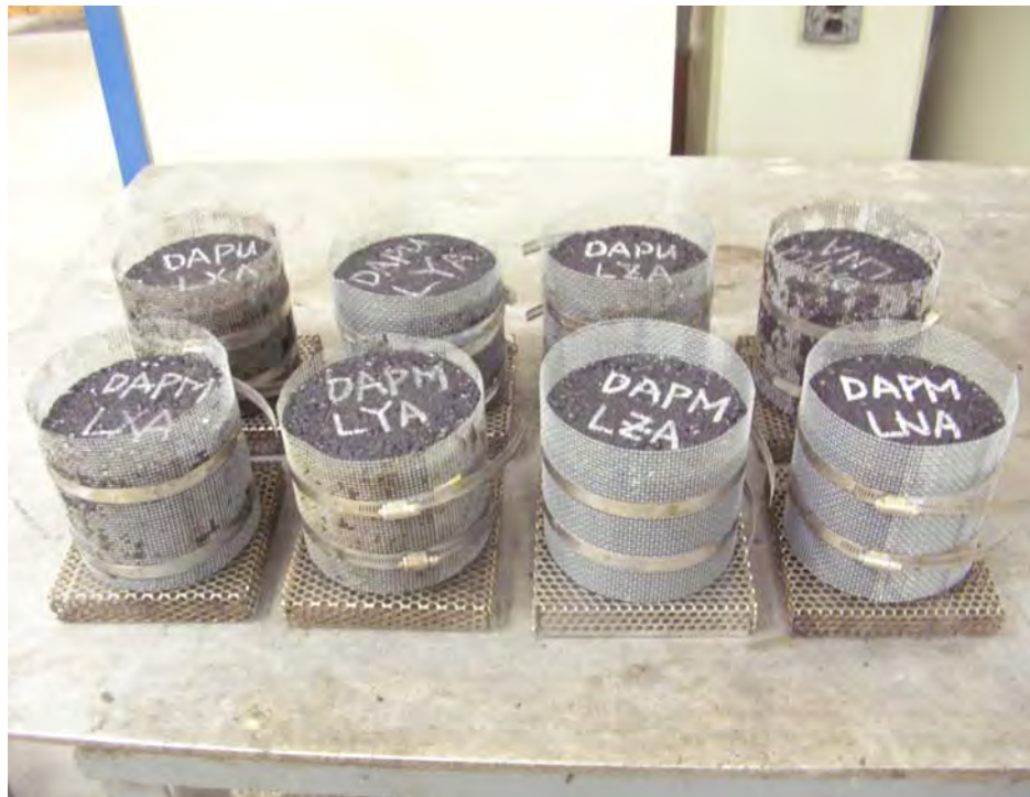
Figure 4-6 Long Term Oven Aging (LTOA) Conditioning Set-up
