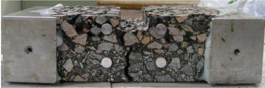
Figure 5-39 Composite Specimen with Rectangular Groove
