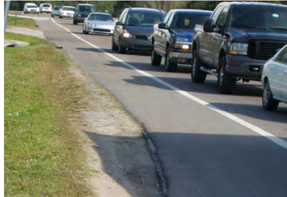
287 - Pasco County, SR 54 at Morris Bridge Road / Eiland Boulevard (CR 579), significant queuing beyond horizontal curve on SR 54 for vehicles approaching intersection from the westbound approach
