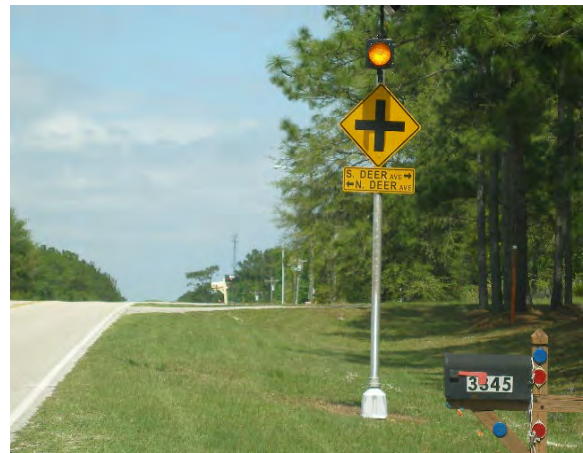
211 - Clay County, CR 215 intersection with Deer Avenue, new high intensity grade warning signs with amber flashing light located at intersections on the crest of a vertical curve where site distances can be a problem
