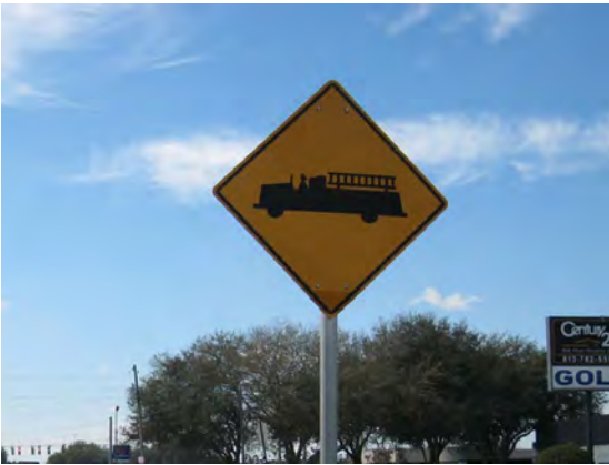
292 - Pasco County, SR 54 at Morris Bridge Road / Eiland Boulevard (CR 579), seeming improper use of fire station sign (no fire stations in vicinity of intersection along SR 54)
