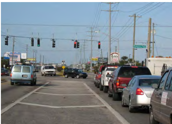
264 - Pasco County, Ridge Road (CR 587) at Regency Boulevard, signal heads for westbound thru vehicles appear to be aligned over painted gore for separated left turn lane
