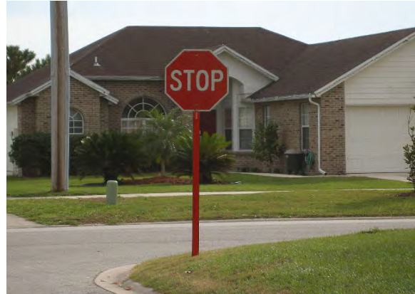
188 - Clay County, Heritage Farms Boulevard at Farm Way, placed reflective red strip on STOP sign post
