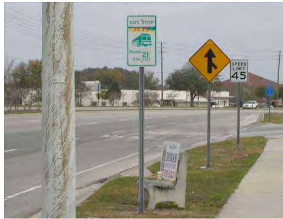
255 - Pasco County, Little Road (CR1) at Embassy Boulevard / Hilltop Drive, bus stop sign on north side limits view of merge sign for northbound vehicles
