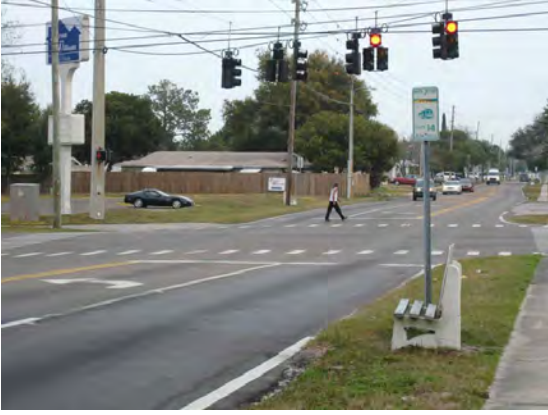
316 - Pasco County, Trouble Creek Road (CR 518) at Madison Street, bus stops do not have concrete landing pads
