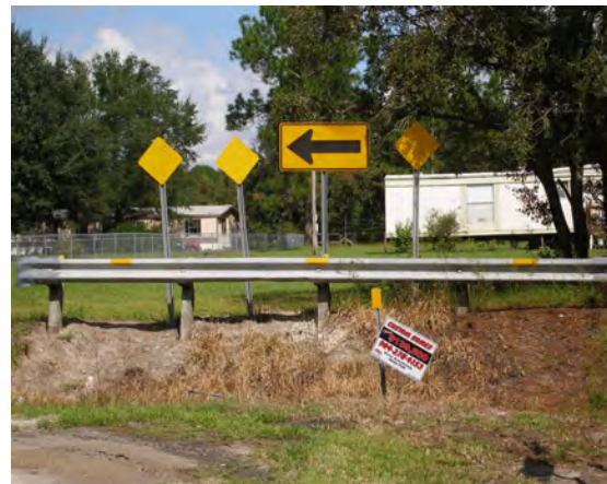
159 - Clay County, Thunder Road north of SR 16, assembly in accordance with FDOT Design Standard Index No. 17349 , Case I
