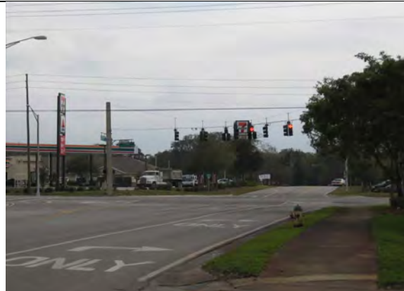
251 - Pasco County, Little Road (CR1) at Embassy Boulevard / Hilltop Drive, north and southbound approaches each have two signal heads serving the three thru lanes
