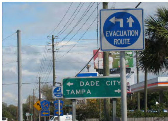
289 - Pasco County, SR 54 at Morris Bridge Road / Eiland Boulevard (CR 579), two different consecutive evacuation signs on eastbound approach, second sign impeding view of county road designation signs
