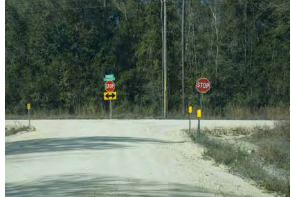
51 – Madison County, traveling southwest on Captain Brown Road approaching Florida Road, double STOP signs added
