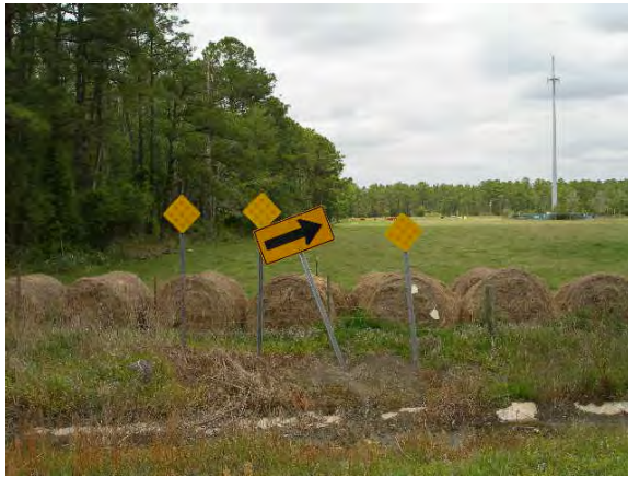
196 - Clay County, Mallard Road ½ mile south of CR 218, assembly following FDOT Design Standard #17349, arrow sign has been pushed and needs straightening
