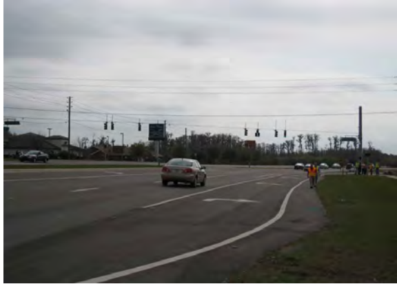
327 - Pasco County, Little Road (CR 1) at Rancho del Rio Drive, no signs indicating name of next signalized intersections along corridor and no street lighting present at intersection
