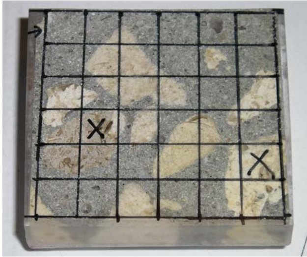
Figure 4-1 Concrete sample with grid
