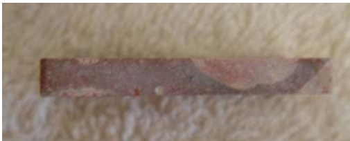
Figure 3-4 Red-dye water-ethanol replacement in control sample
