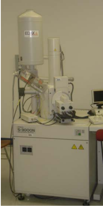
Figure 4-2 Hitachi S-3000N SEM from the University of Florida Advanced Material Characteristic Lab
