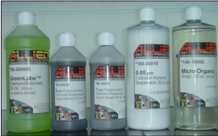
Figure 3-9 Consumables from Allied High Tech, Inc. used for grinding/polishing
