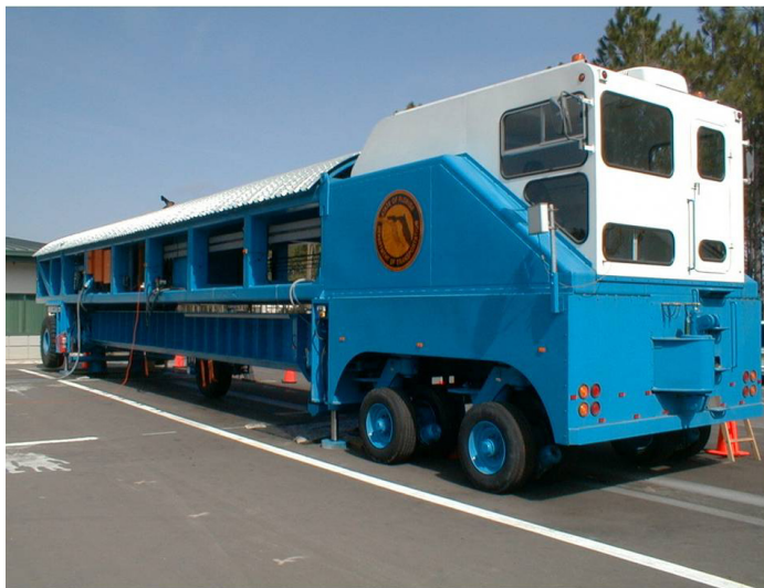
The heavy vehicle simulator was used to test artificially aged pavement.
