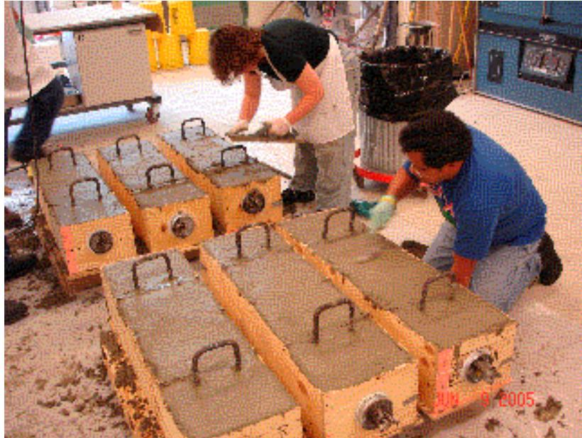
**Figure 5. FDOT and UF Personnel Finish Concrete in Slab Forms.**
