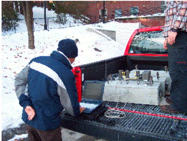
**Figure 8. IE Testing in Progress.**
