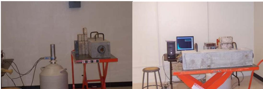
**Figure 11. The Experimental Setup for Measuring the 2.22 MeV Gamma-ray from Neutron Capture with Hydrogen.**
