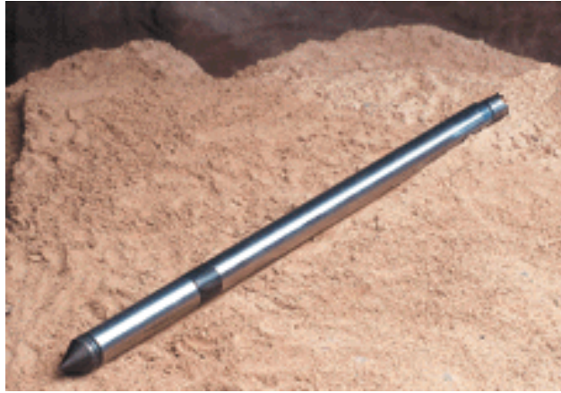
Figure 2-1. Conventional cone penetrometer
