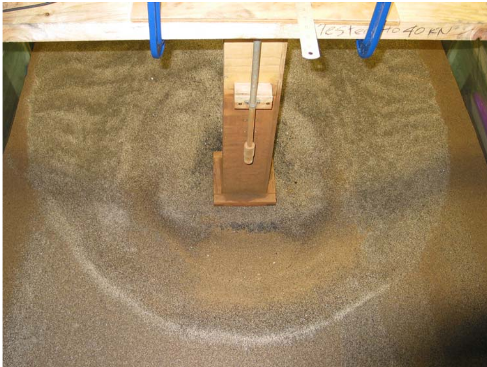
Figure 29 Post Scour Test 2 Photograph Taken From Above and Upstream.
