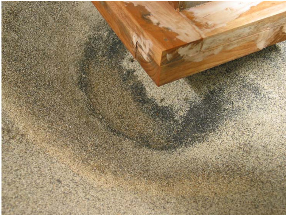
Figure 61 Post Scour Test 7 Photograph Taken From Above.
