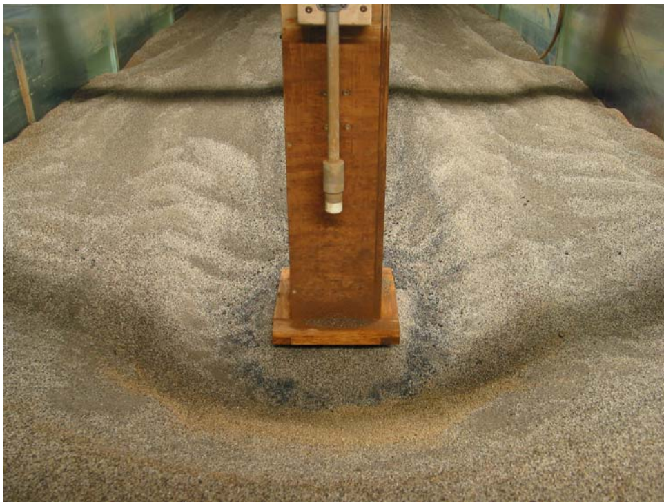
Figure 21 Post Scour Test 1 Photograph Taken From Upstream.
