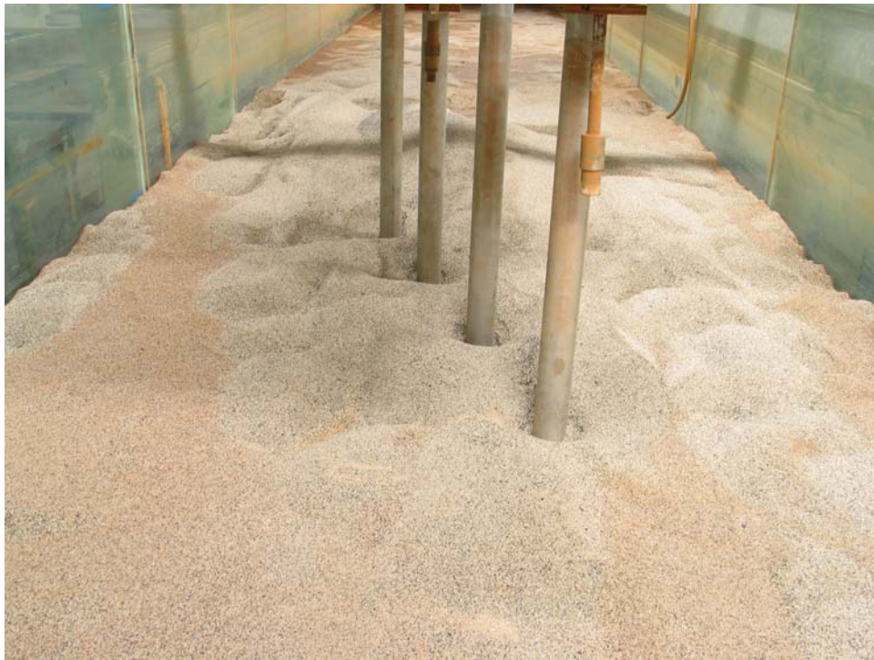
Figure 53 Post Scour Test 6 Photograph Taken From Upstream.
