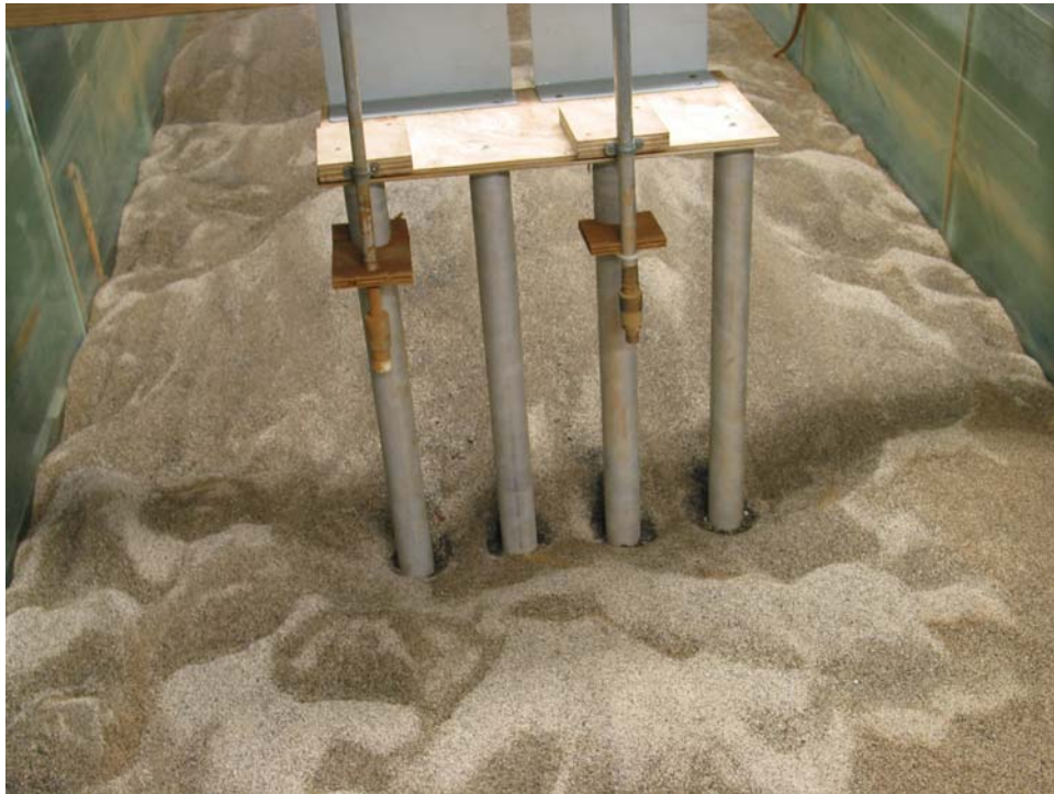
Figure 41 Post Scour Test 4 Photograph Taken From Upstream.
