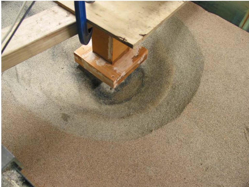
Figure 59 Post Scour Test 7 Photograph Taken From Upstream.
