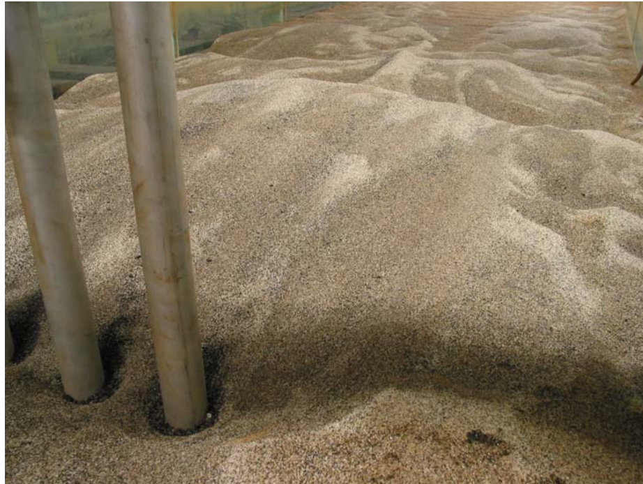
Figure 43 Post Scour Test 4 Photograph Taken of the Downstream Bed.
