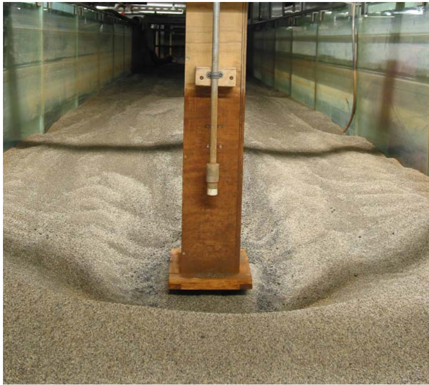
Figure 24 Post Scour Test 1 Photograph Taken From Upstream.
