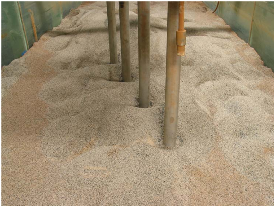
Figure 56 Post Scour Test 6 Photograph Taken From Upstream.
