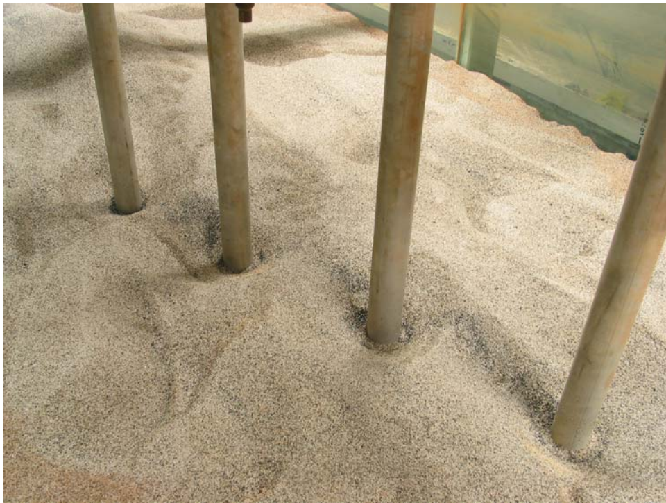
Figure 55 Post Scour Test 6 Photograph Taken From Above.
