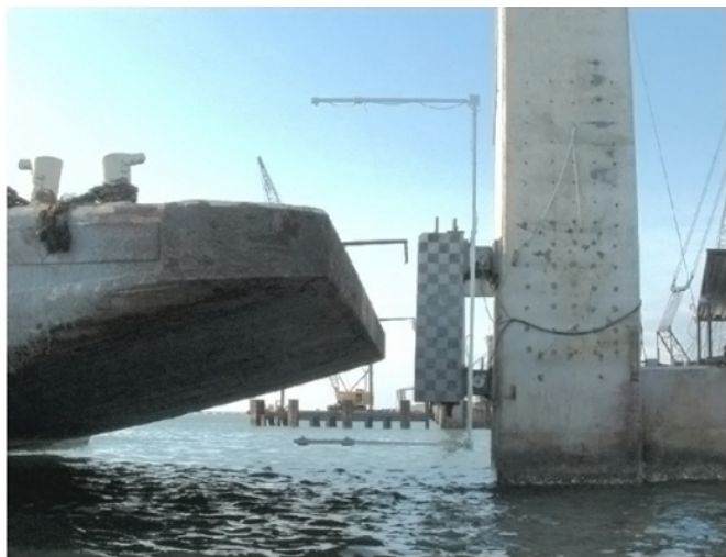
The dynamic model is based on extensive real life barge impact tests.
