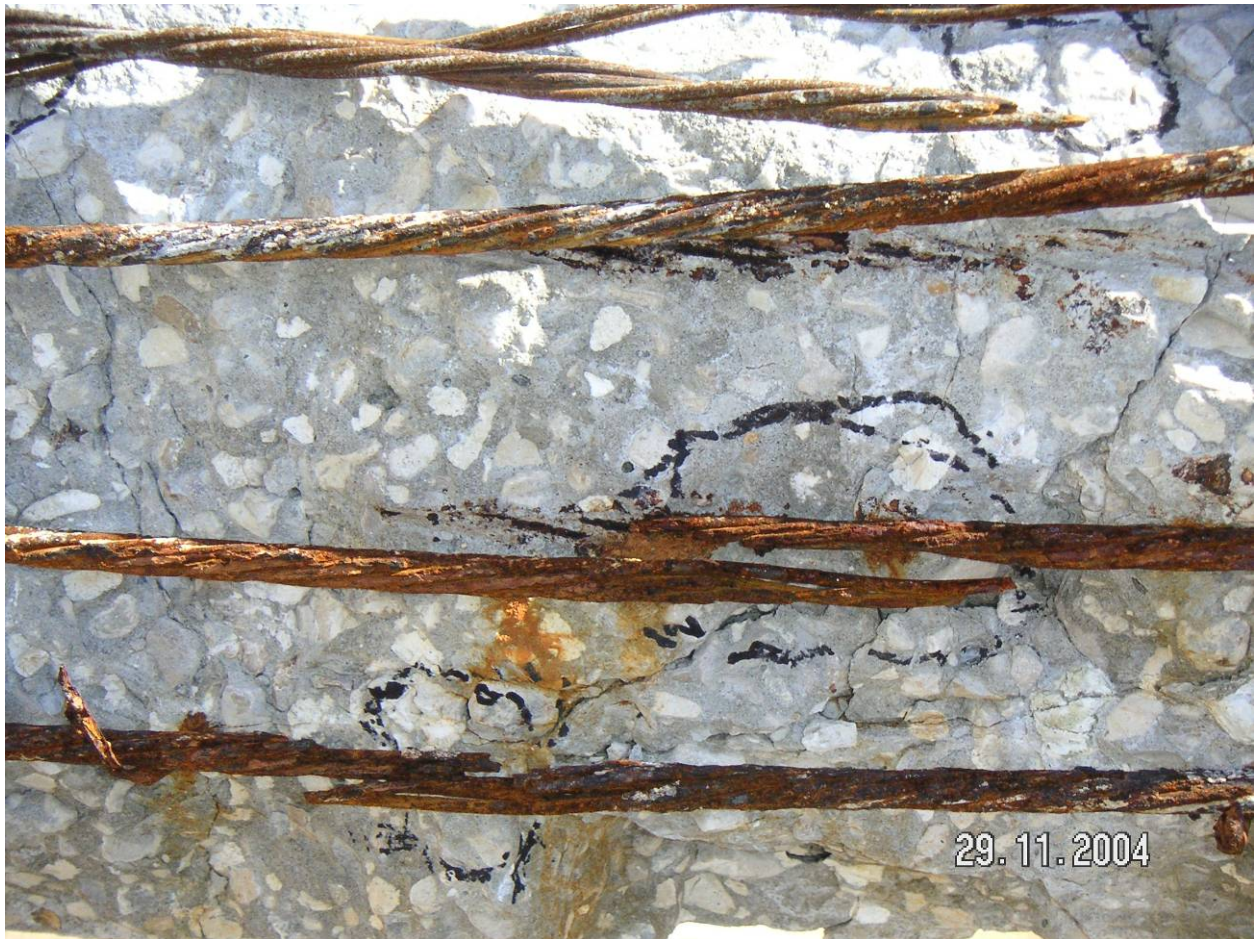
Figure 32 – Strand in bottom of pile 44-3CP. Corrosion severity increases in intensity from top to bottom. Wire breaks are distributed along a major flexural crack in the more heavily corroded strands.
