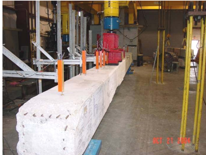
Figure 16 – Instrumentation for flexural testing
