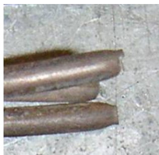
Figure 34 – Failure mode of uncorroded prestressing strand sample taken from pile 44-2. Ductile necking of the cross section and cup/cone fracture surface are shown.
