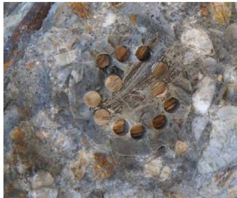
Figure 40 – Prestressing tendon from cylinder pile. Note grout surrounding wire with no evidence of conduit.
