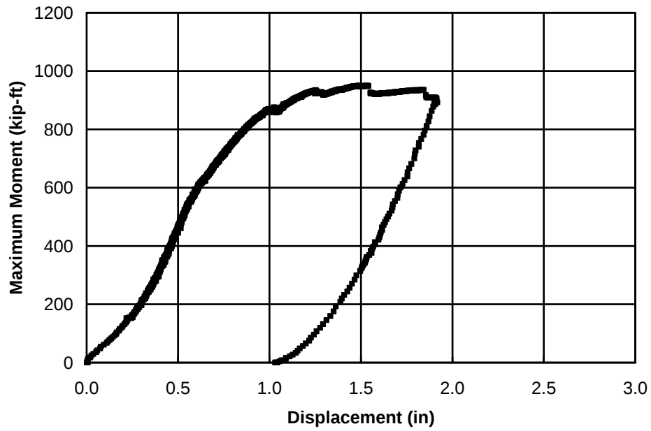
Figure 43 – Load deflection response CP2
