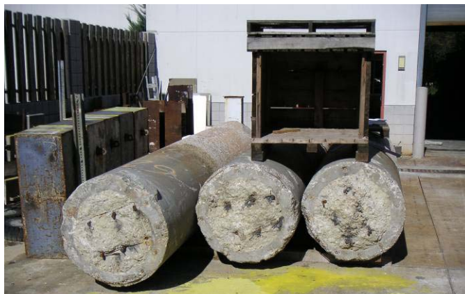
Figure 38 – Three piles prior to testing, view of filled end of pile.
