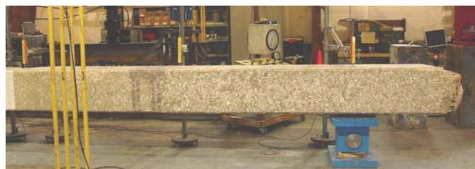
Figure 18 – DT placement at pile ends
