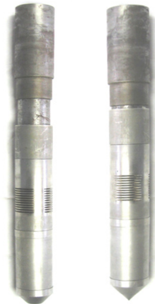
The VAHIP Probe, showing the Stage I vertical permeability test mode position on the right and the Stage II horizontal permeability test mode position on the left
