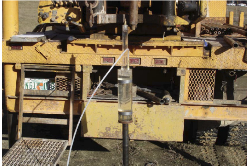
Vertical and Horizontal Insitu Permeameter (VAHIP) Probe
